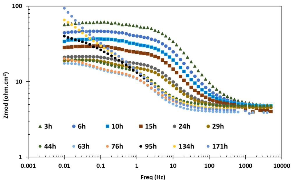
Figure 108. Impedance modulus. EIS spectra obtained over time from a baseline experiment ( $S_{CaCO_3} = 0$ ) conducted at 80°C,  $pCO_2$  0.53 bar, bulk solution pH 5.5, 0.60 M ionic strength, and 20 rpm
