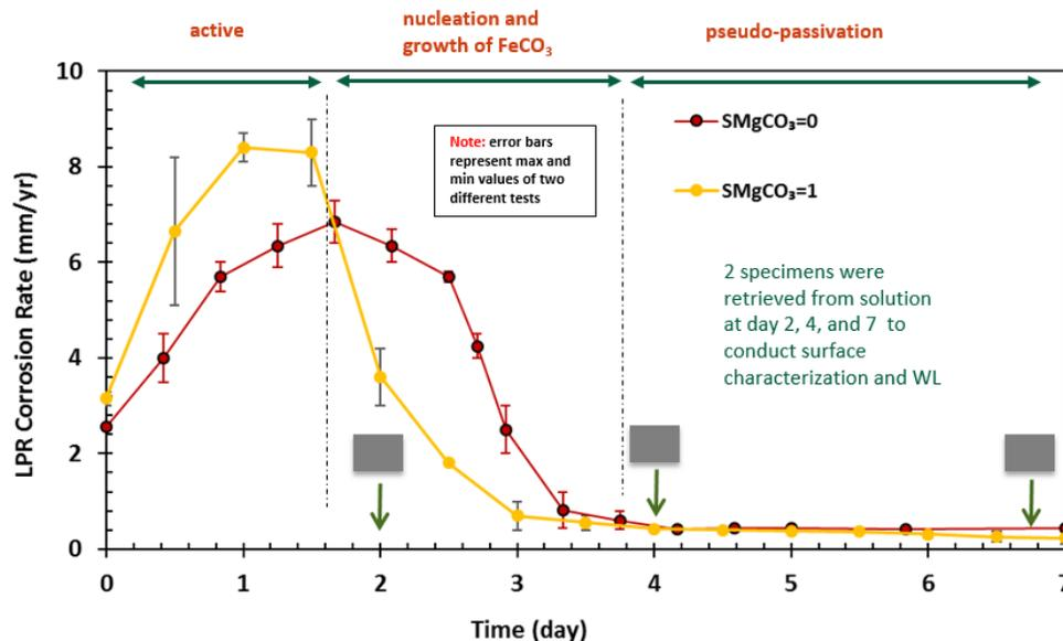
Figure 79. Trend of corrosion rate obtained by LPR over time with and without the presence of 100 ppm Mg<sup>2+</sup> at pH 6.2
