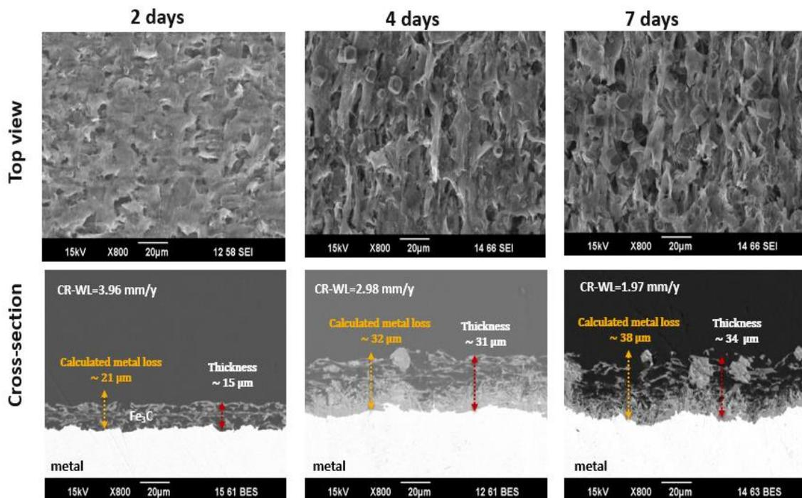
Figure 32. Top and cross-sectional views of specimens retrieved from the test condition with  $\text{CaCO}_3$  present after 2, 4 and 7 days of exposure at pH 6.2
