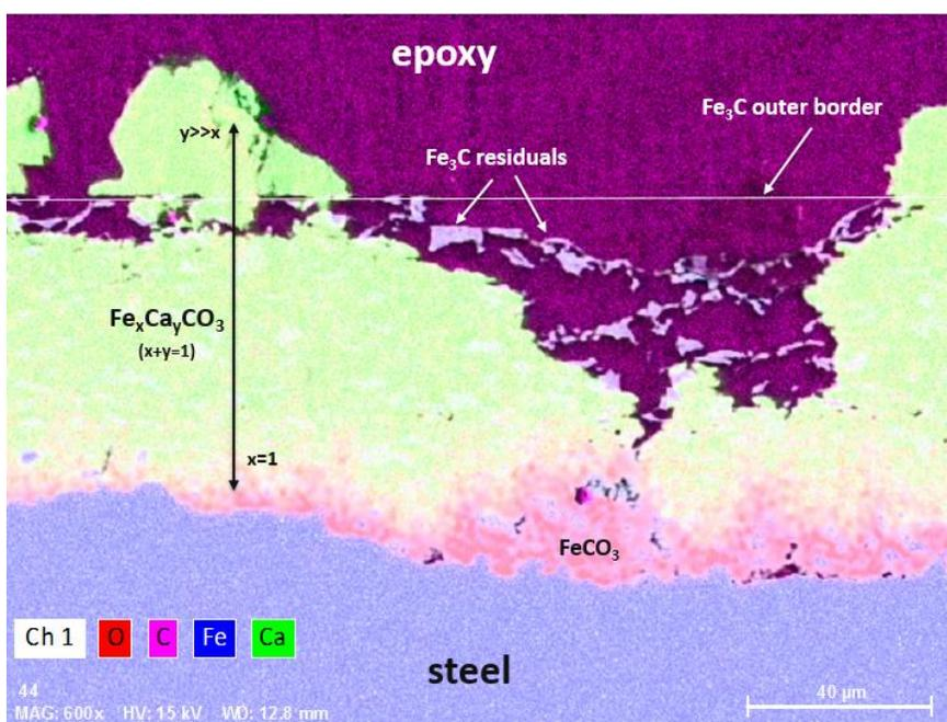
Figure 46. EDS analysis (map mode) of a cross-section UNS G10180 specimen after 7 days of exposure to a  $\text{CaCO}_3$ -saturated solution at  $80^\circ\text{C}$ , bulk solution pH 5.5,  $\text{pCO}_2$  0.53 bar, 0.60 M ionic strength, and 6000 ppm  $\text{Ca}^{2+}$
