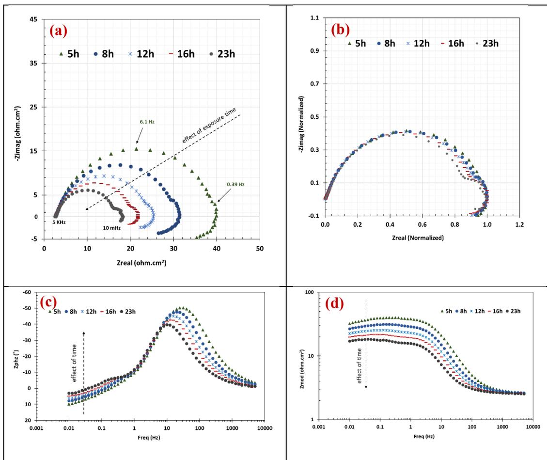
Figure 114. EIS results obtained from active corrosion period of an experiment with presence of  $6000 \text{ ppm Ca}^{2+}$  ( $S_{CaCO_3} = 1$ ) conducted at  $80^\circ\text{C}$ ,  $p\text{CO}_2$  0.53 bar, bulk solution pH 5.5, 0.60 M ionic strength, and 20 rpm: (a) Nyquist plots (b) normalized Nyquist plots (c) phase angle, and (d) impedance modulus
