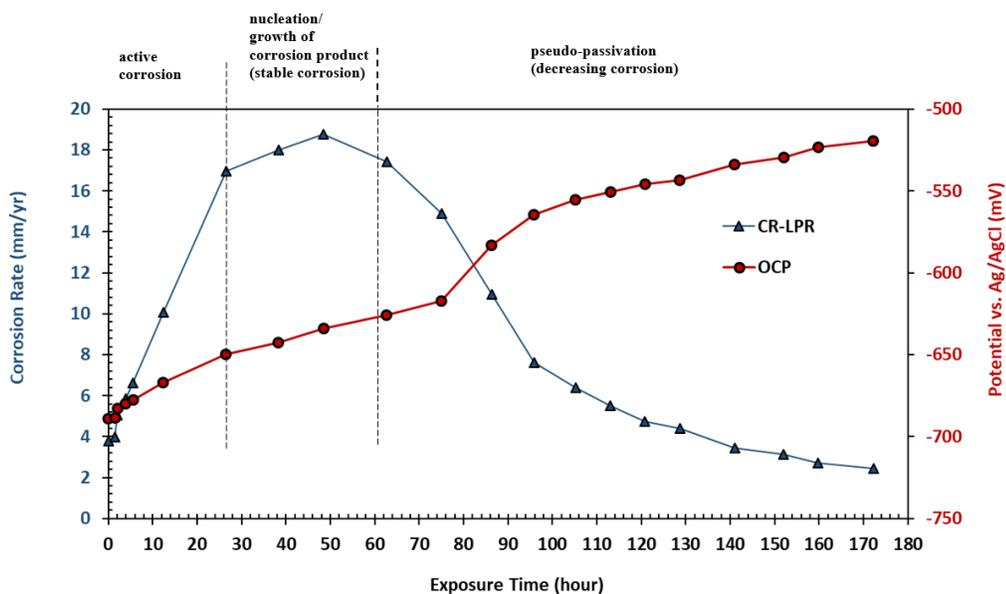
Figure 105. LPR corrosion rate and OCP variation over time for a baseline experiment ( $S_{\text{CaCO}_3} = 0$ ) conducted at  $80^\circ\text{C}$ ,  $p\text{CO}_2$  0.53 bar, bulk solution pH 5.5, 0.60 M ionic strength, and 20 rpm
