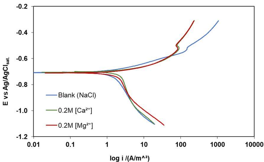
Figure 120. Potentiodynamic polarization of mild steel in presence of a blank, Ca<sup>2+</sup>-containing, and Mg<sup>2+</sup>-containing solution at 40°C, pCO<sub>2</sub> 0.93 bar, bulk solution pH 4.64, 0.77 M ionic strength, and 1500 rpm
