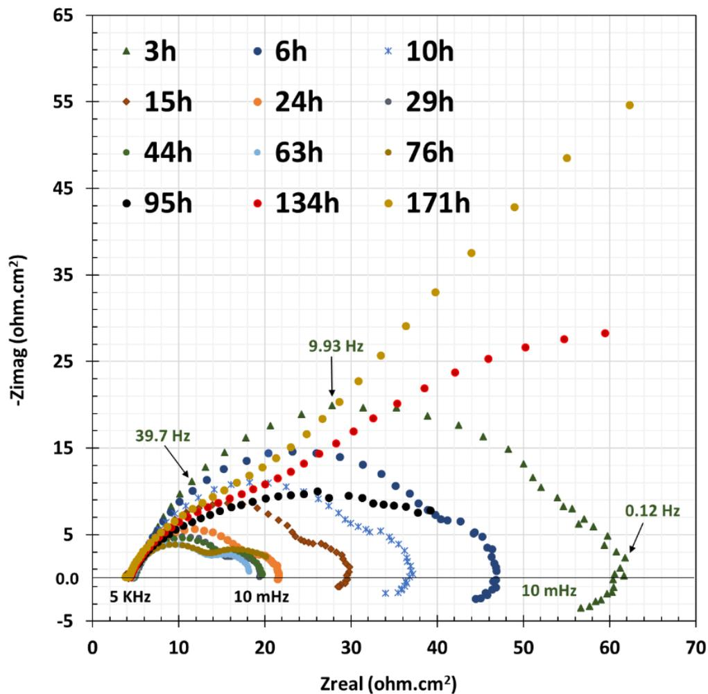
Figure 106. Nyquist plot. EIS spectra obtained over time from a baseline experiment ( $S_{\text{CaCO}_3} = 0$ ) conducted at OCP at 80°C, pCO<sub>2</sub> 0.53 bar, bulk solution pH 5.5, 0.60 M ionic strength, and 20 rpm
