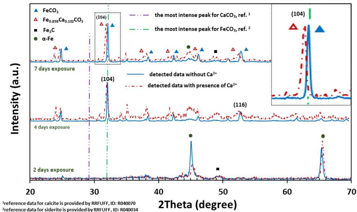
Figure 34. XRD patterns of surface layers detected on the steel surface after 2, 4, and 7 days of exposure with/without the presence of  $\text{Ca}^{2+}$  at pH 6.2
