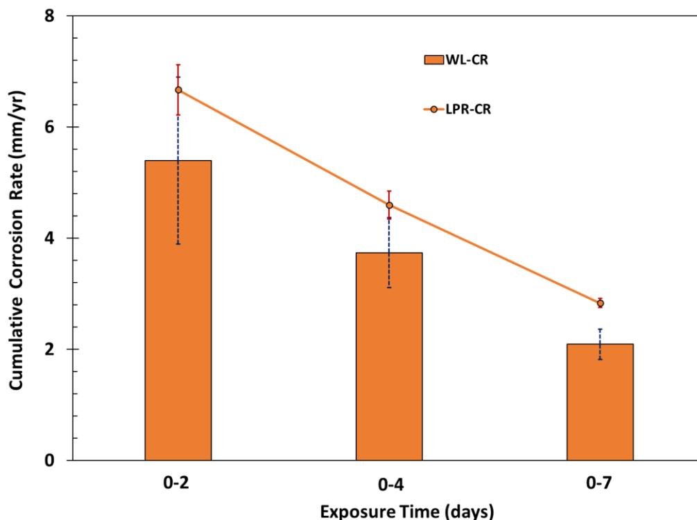
Figure 22. Time-averaged (cumulative) corrosion rate obtained by LPR and WL techniques (UNS G10180, 80 °C,  $p\text{CO}_2$  0.53 bar, pH 6.2, NaCl 1wt%,  $4 < S_{FeCO_3} < 14$ ,  $S_{CaCO_3} = 0$ , velocity 0.58 m/s)
