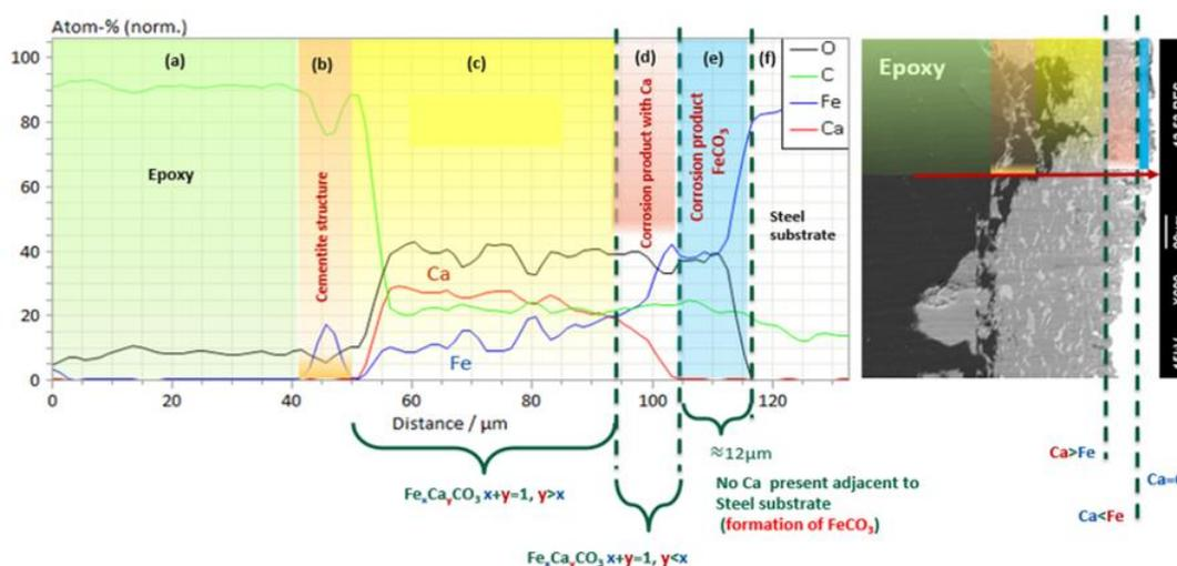
Figure 45. EDS analysis (line scan) of the surface layers formed on carbon steel after 7 days of exposure to a solution with the presence of 6000 ppm  $\text{Ca}^{2+}$  ( $S_{\text{CaCO}_3} = 1$ ) at 80°C,  $\text{pCO}_2$  0.53 bar, bulk solution pH 5.5, 0.60 M ionic strength, and 20 rpm
