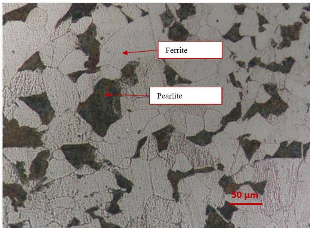
Figure 20. Ferritic-pearlitic microstructure of the UNS G10180 mild steel specimens
