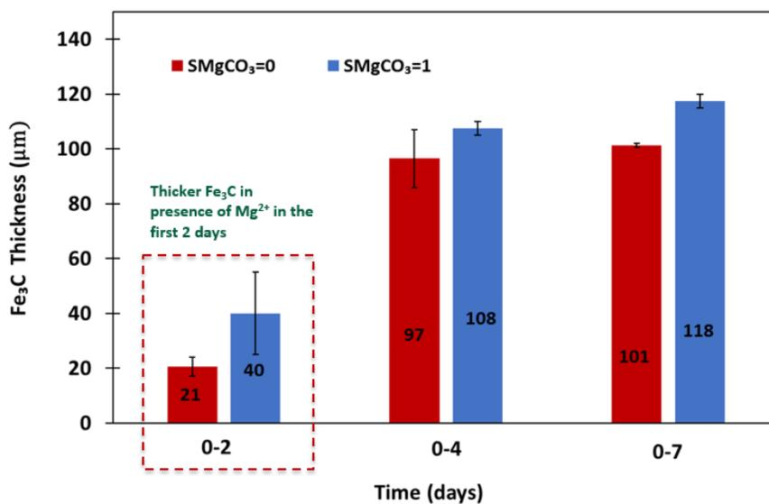
Figure 89. Evolution of Fe<sub>3</sub>C over time with and without presence of 4,200 Mg<sup>2+</sup> (80°C, pCO<sub>2</sub> 0.53 bar, 0.58 m/s, pH 5.5, ionic strength 0.6 M, 1 wt.% NaCl)
