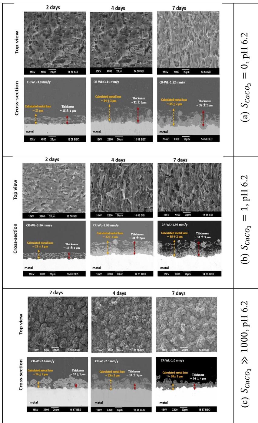
Figure 64. SEM images (top and cross-section view) of the development of surface layers over time for the experiment with different  $CaCO_3$ -saturation level at 80°C,  $pCO_2$  0.53 bar, 20rpm, pH 6.2, ionic strength 0.18 M
