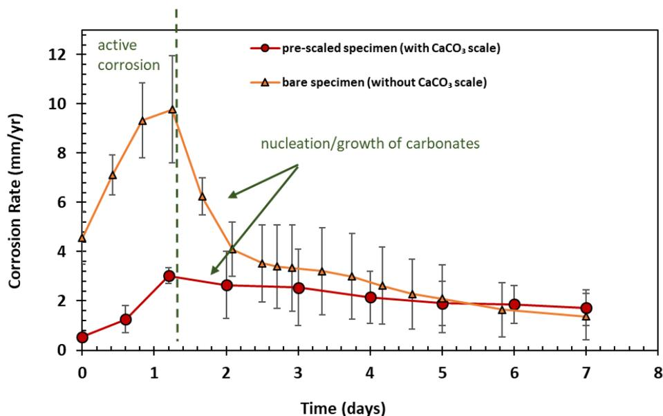
Figure 57. Comparison of corrosion behavior of mild steel with and without  $\text{CaCO}_3$  scale at bulk solution pH 5.5,  $80^\circ\text{C}$ , 0.53 bar  $\text{pCO}_2$ , ionic strength 0.6M, 6000 ppm  $\text{Ca}^{2+}$  ( $S_{\text{CaCO}_3} = 1$ ), and 20 rpm
