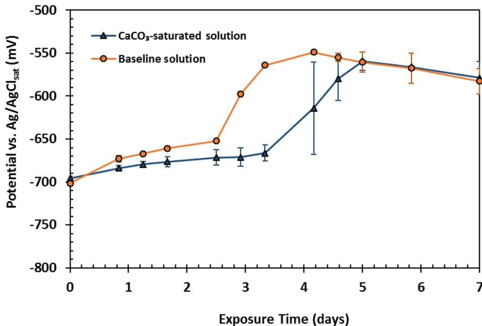
Figure 31. Comparison of OCP over time for UNS G10180 exposed to solutions with and without CaCO<sub>3</sub> at pH 6.2
