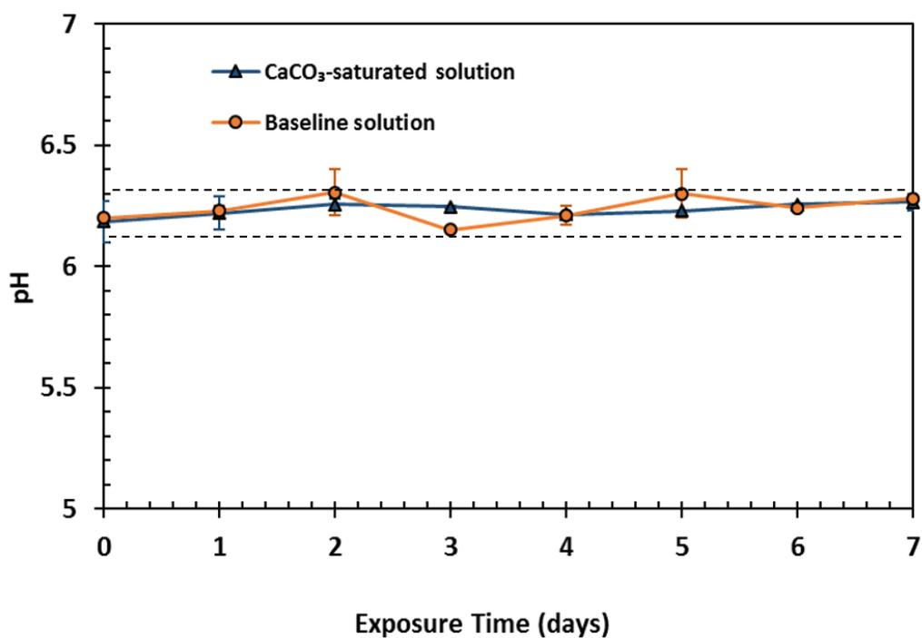
Figure 27. pH profiles for both baseline and  $\text{CaCO}_3$ -saturated solution over time (pH  $6.2 \pm 0.1$ )
