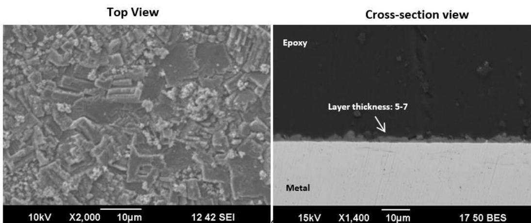
Figure 49. Top and cross-section view SEM of the surface layers formed on the steel during 5 days of cathodic polarization;  $\text{CaCO}_3$ -saturated solution (6000 ppm  $\text{Ca}^{2+}$ ),  $80^\circ\text{C}$ , bulk solution pH 5.5,  $\text{pCO}_2$  0.53 bar, 0.60 M ionic strength, 20 rpm
