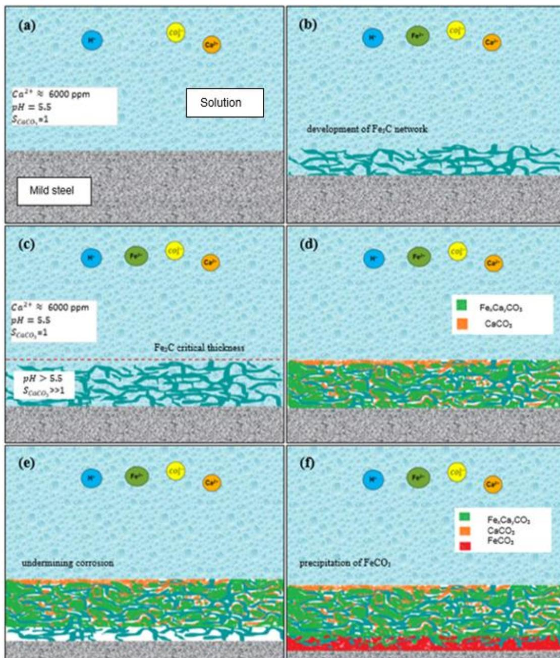
Figure 48. A descriptive model for CO<sub>2</sub> corrosion mechanism of mild steel exposed to the CaCO<sub>3</sub>-saturated solution at 80°C, bulk solution pH 5.5, pCO<sub>2</sub> 0.53 bar, 6000 ppm Ca<sup>2+</sup>, 0.60 M ionic strength, and 20 rpm
