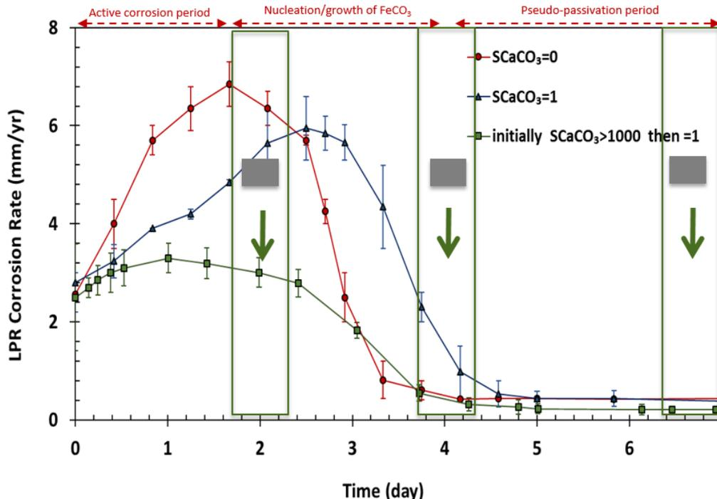
Figure 61. Comparison of LPR corrosion behavior of UNS G10180 exposed to solutions with different  $CaCO_3$  saturation levels ( $80^\circ C$ ,  $pCO_2$  0.53 bar, 20 rpm, pH 6.2, ionic strength 0.18 M,  $[Ca^{2+}] \sim 160$  ppm)
