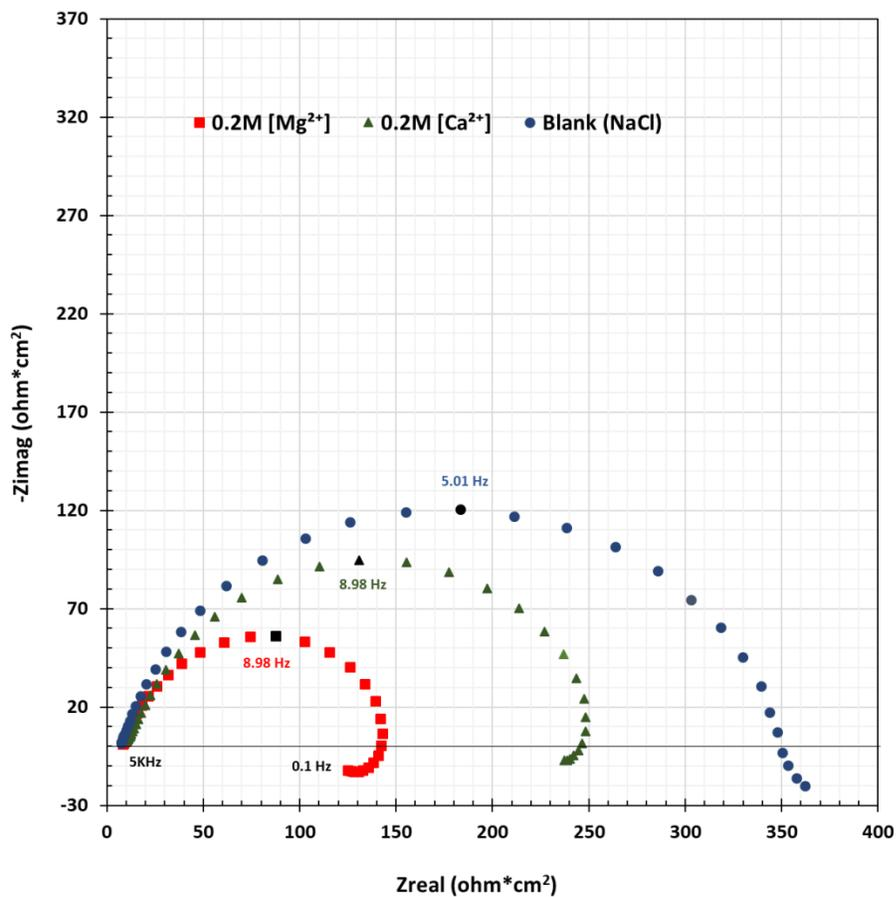
Figure 117. Nyquist plots obtained from a blank, Ca<sup>2+</sup>-containing, and Mg<sup>2+</sup>-containing solution at 40°C, pCO<sub>2</sub> 0.93 bar, bulk solution pH 4.64, 0.77 M ionic strength, and 1500 rpm
