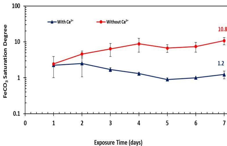
Figure 37. Variation of  $\text{FeCO}_3$  saturation degree over time for the experiments with and without 6000 ppm  $\text{Ca}^{2+}$  ( $S_{\text{CaCO}_3} = 1$ ) at  $80^\circ\text{C}$ ,  $\text{pCO}_2$  0.53 bar, bulk solution pH 5.5, 0.60 M ionic strength, and 20 rpm
