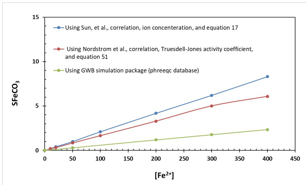
Figure 104. Effect of non-ideality: comparison of iron carbonate saturation ( $S_{FeCO_3}$ ) calculation using Equation 17, Equation 51, and GWB simulation at 80°C,  $pCO_2$  0.53 bar, bulk solution pH 5.5, 0.60 M ionic strength
