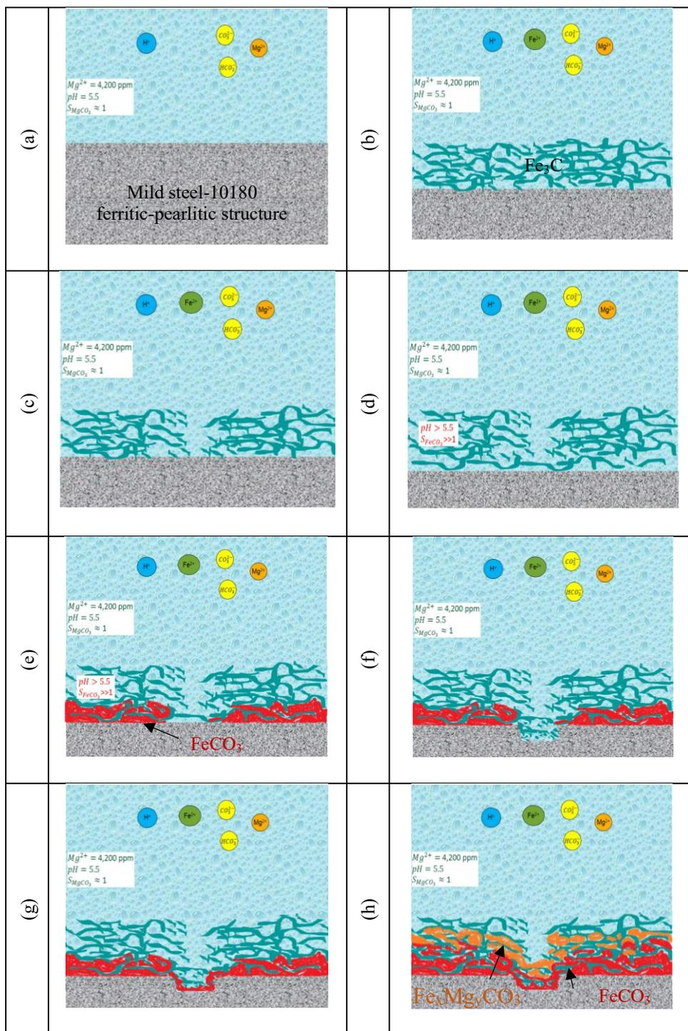
Figure 95. Proposed mechanism for the localized corrosion observed in presence of high  $[Mg^{2+}]$  for mild steel at 4,200 ppm  $Mg^{2+}$ ,  $80^\circ C$ ,  $pCO_2$  0.53 bar, 0.58 m/s, pH 5.5, ionic strength 0.6M, 1 wt.% NaCl
