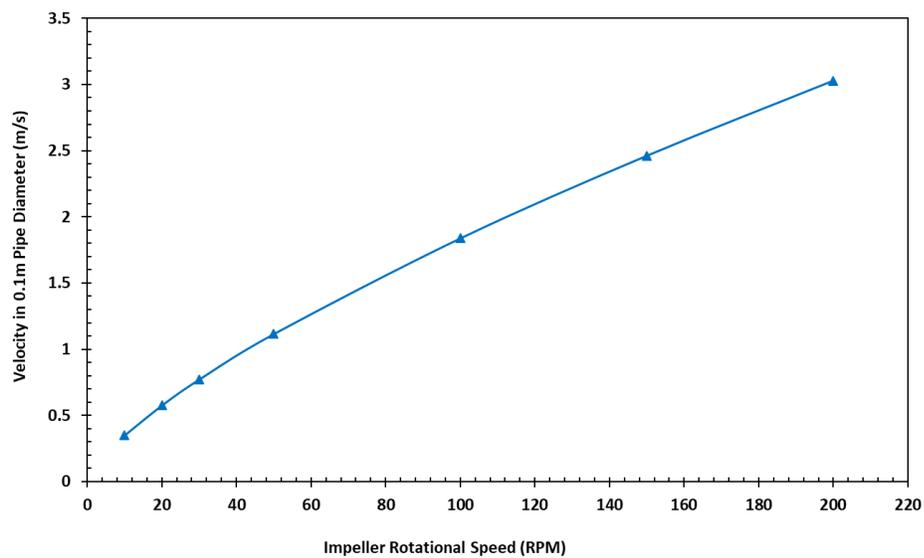
Figure 19. The relation between impeller rotational speed in the glass cell and velocity of the fluid in single-phase flow through a 0.1m ID pipe obtained by matching mass transfer coefficients.
