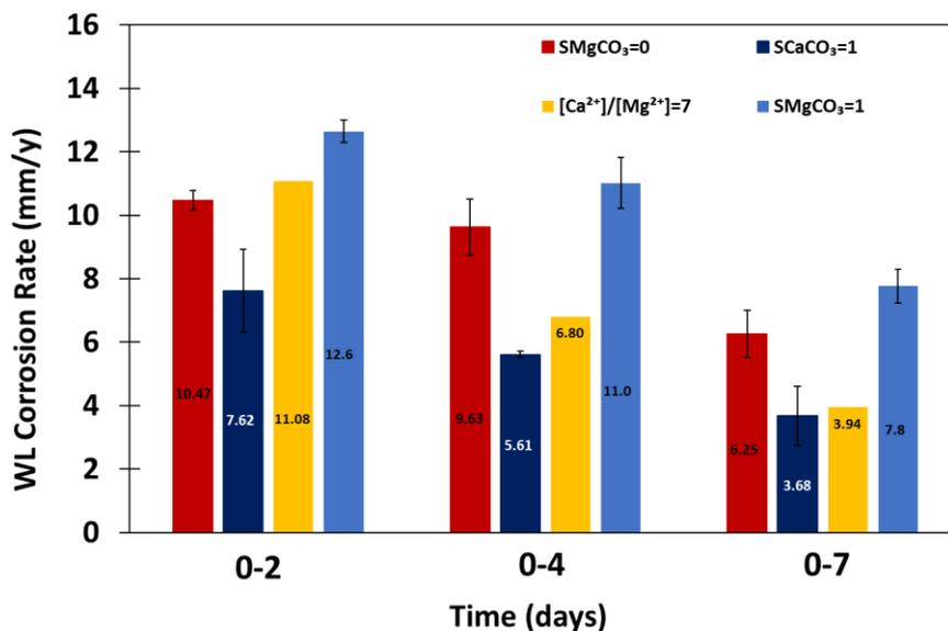
Figure 97. Cumulative corrosion rate obtained by WL over time at 80°C, pCO<sub>2</sub> 0.53 bar, 0.58 m/s, pH 5.5, ionic strength 0.6M [baseline (red), 6000 ppm Ca<sup>2+</sup> (dark blue), Ca<sup>2+</sup>/Mg<sup>2+</sup>=7 (yellow), and 4200 ppm Mg<sup>2+</sup> (light blue)]
