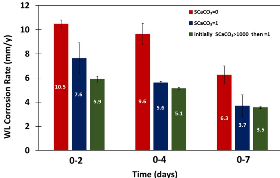
Figure 72. Cumulative corrosion rate by weight loss technique over time for solutions with different CaCO<sub>3</sub> saturation level at 80°C, pCO<sub>2</sub> 0.53 bar, 20 rpm, pH 5.5, ionic strength 0.6 M, [Ca<sup>2+</sup>] ~6000 ppm
