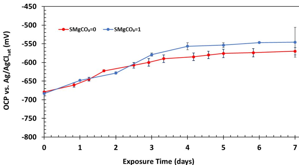
Figure 90. Comparison of OCP over time for UNS G10180 exposed to solutions with and without 4,200 ppm Mg<sup>2+</sup> (80°C, pCO<sub>2</sub> 0.53 bar, 0.58 m/s, pH 5.5, ionic strength 0.6 M, 1 wt.% NaCl)
