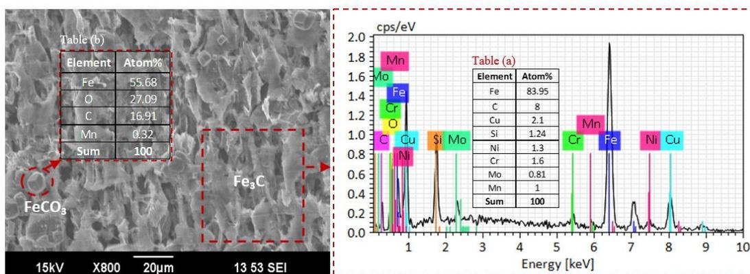
Figure 26. SEM/EDS analysis (top view) of the corrosion products developed on the surface of UNS G10180 specimens exposed to the baseline solution for 7 days at pH 6.2
