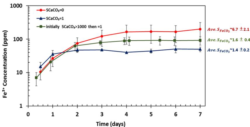
Figure 70. Variation of  $[Fe^{2+}]$  over time for the experiments with different  $CaCO_3$  saturation level at  $80^\circ C$ ,  $pCO_2$  0.53 bar, 20 rpm, pH 5.5, ionic strength 0.6 M,  $[Ca^{2+}] \sim 6000$  ppm
