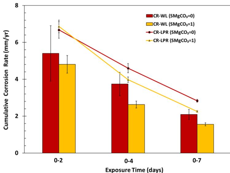
Figure 80. Cumulative corrosion rate by WL (bar chart) and LPR (line chart) techniques over time for solution with and without 100 ppm Mg<sup>2+</sup> (80°C, pCO<sub>2</sub> 0.53 bar, 0.58 m/s, pH 6.2, ionic strength 0.18 M, 1 wt.% NaCl)
