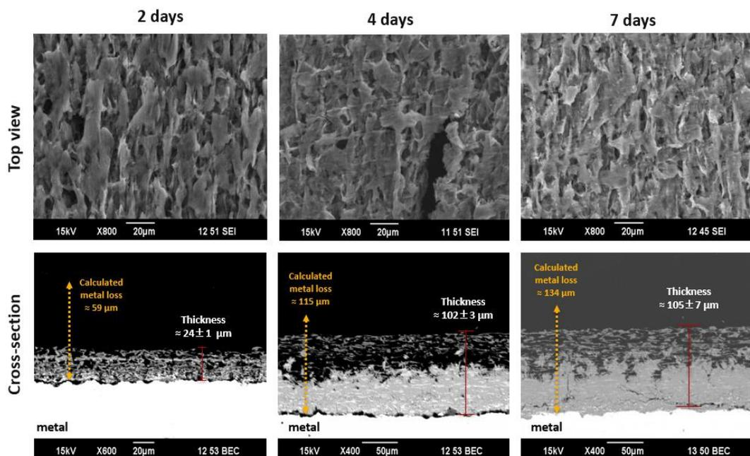
Figure 41. SEM images (top and cross-section view) of the development of surface layers over time for the experiment without  $\text{Ca}^{2+}$  at  $80^\circ\text{C}$ ,  $\text{pCO}_2$  0.53 bar, bulk solution pH 5.5, 0.60 M ionic strength, and 20 rpm
