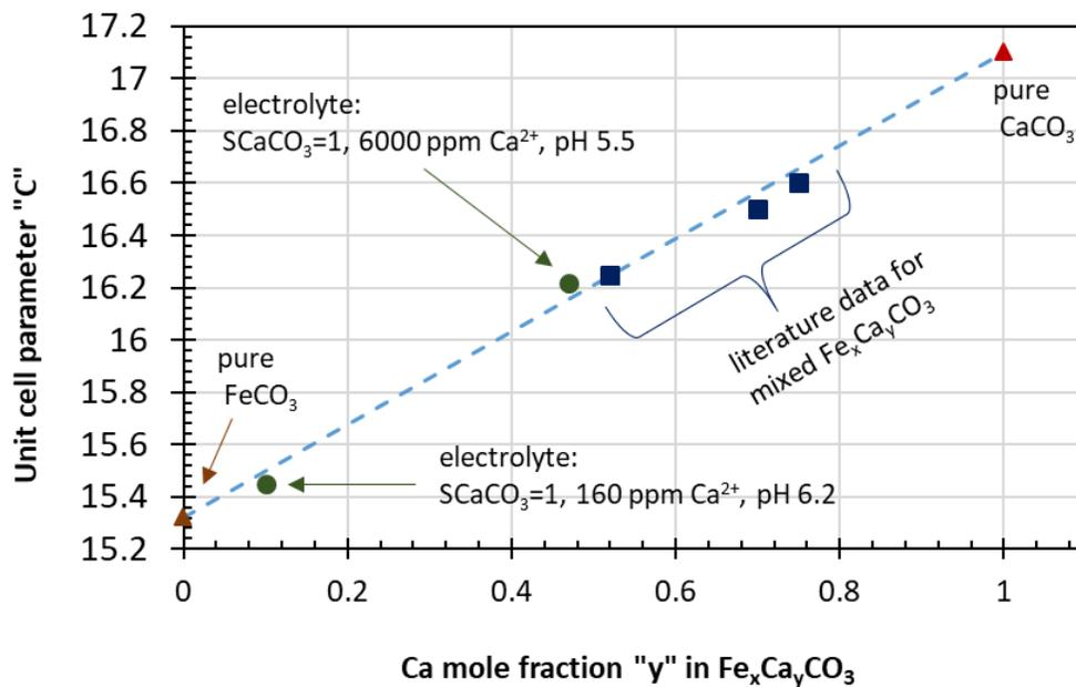
Figure 102. Unit cell parameter "c" versus the Ca mole fraction in the lattice of mixed  $Fe_xCa_yCO_3$  for the  $CaCO_3$ -saturated solutions with 160 and 6000 ppm dissolved  $Ca^{2+}$  at pH 6.2 and 5.5, respectively
