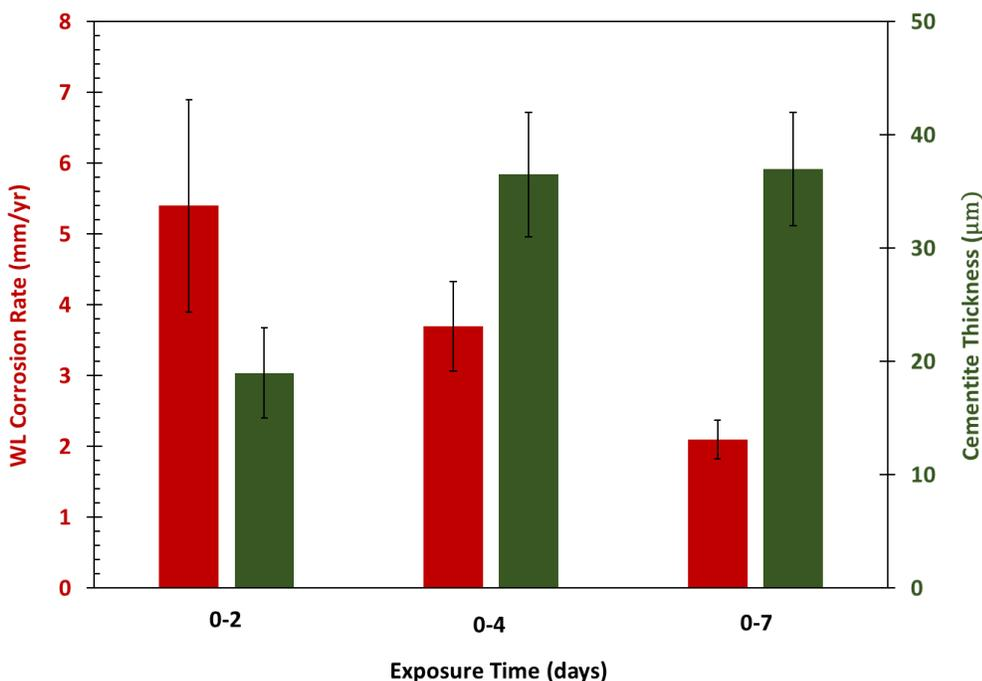
Figure 24. Corrosion rate by WL and cementite thickness *versus* time in the active (2 days), nucleation/growth of  $\text{FeCO}_3$  (4 days), and pseudo-passive (7 days) periods, baseline experiment at pH 6.2.
