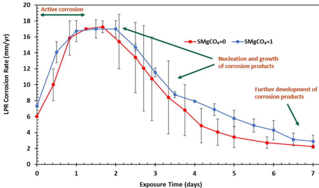
Figure 87. Trend of corrosion rate obtained by LPR over time with and without presence of 4,200 ppm Mg<sup>2+</sup> at pH 5.5
