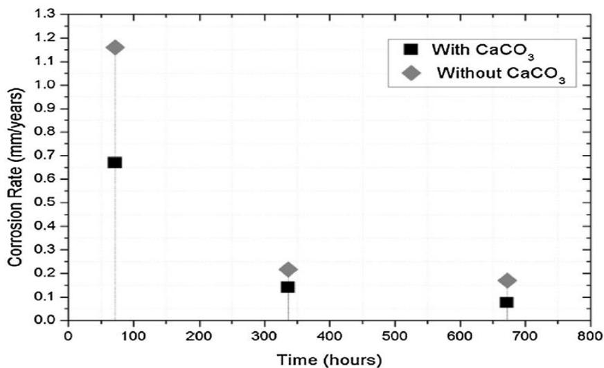
Figure 14. Corrosion rate, by weight loss, *versus* exposure time for test electrolytes with and without CaCO<sub>3</sub> at 80°C, pCO<sub>2</sub> 15 MPa, solution saturated with CO<sub>2</sub> and NaCl (reproduced with permission [50])
