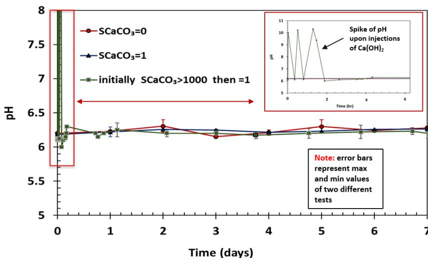
Figure 59. Variation of bulk solution pH over time for the experiments with different  $\text{CaCO}_3$  saturation levels ( $80^\circ\text{C}$ ,  $p\text{CO}_2$  0.53 bar, 20 rpm, ionic strength 0.18 M,  $[\text{Ca}^{2+}] \sim 160$  ppm)
