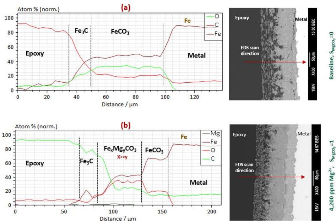
Figure 92. EDS line scan analysis of the surface layers developed on the specimens after 7 days of exposure to electrolytes without (a) and with (b) 4,200 ppm  $\text{Mg}^{2+}$  at  $80^\circ\text{C}$ ,  $\text{pCO}_2$  0.53 bar, 0.58 m/s, pH 5.5, ionic strength 0.6 M, 1 wt.% NaCl
