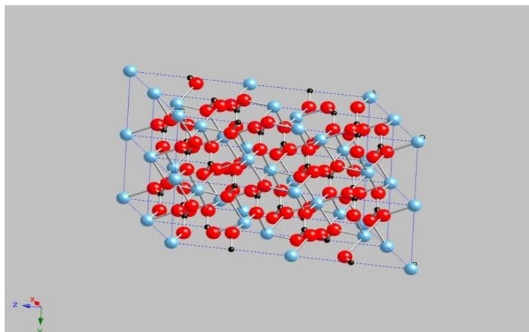
Figure 2. Hexagonal crystal structure of calcite ( $\text{CaCO}_3$ ; blue = Ca, red = O, black =C), four-unit cells
