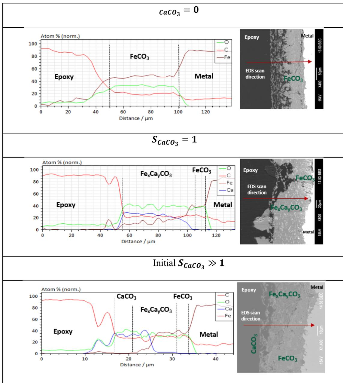
Figure 76. EDS line scan analysis of the surface layers developed on the specimen after 7 days of exposure to electrolytes with different  $CaCO_3$  saturation level at  $80^\circ C$ ,  $pCO_2$  0.53 bar, 20 rpm, pH 5.5, ionic strength 0.6 M,  $[Ca^{2+}] \sim 6000$  ppm.
