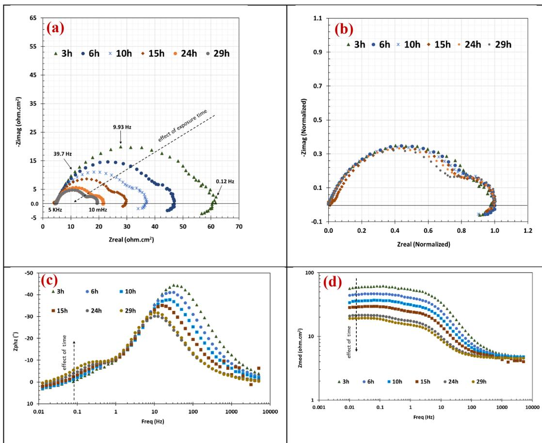
Figure 109. EIS results obtained from active corrosion period of a baseline experiment ( $S_{CaCO_3} = 0$ ) conducted at 80°C,  $pCO_2$  0.53 bar, bulk solution pH 5.5, 0.60 M ionic strength, and 20 rpm: (a) Nyquist plots (b) normalized Nyquist plots (c) phase angle, and (d) impedance modulus
