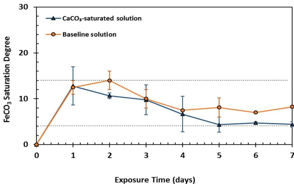
Figure 28. Variation of  $\text{FeCO}_3$  saturation degree over time for experiment with and without  $\text{CaCO}_3$  at pH 6.2 (the average values of  $S_{\text{FeCO}_3}$  were controlled between 4 and 14)
