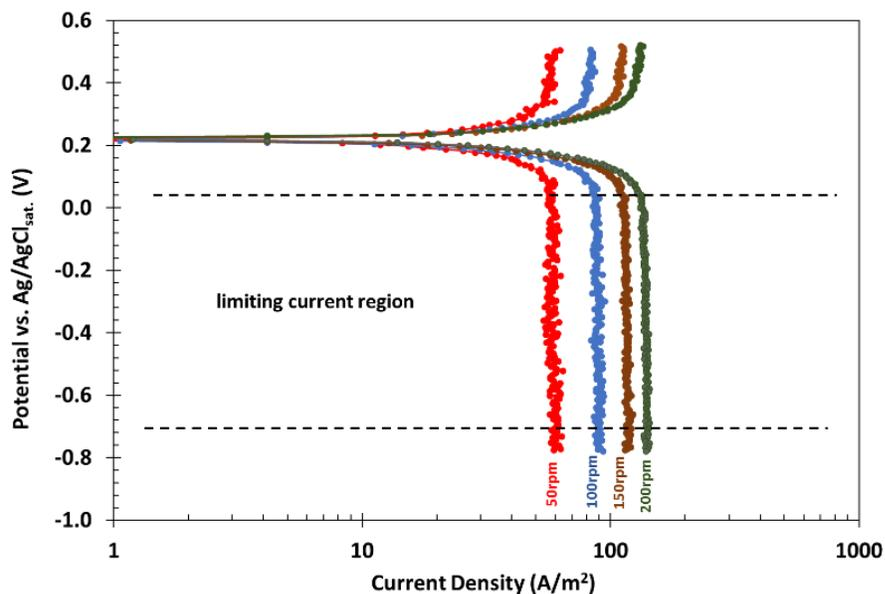
Figure 17. Limiting currents obtained at 50°C and varying rotational speeds using ferri-ferrocyanide coupled reactions
