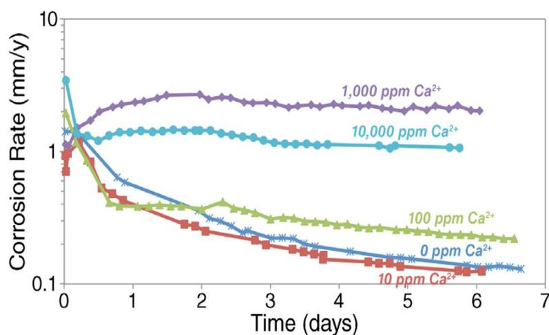
Figure 11. Corrosion rate over time measured by LPR for different initial concentration of calcium ions at  $80^\circ\text{C}$ ,  $\text{pCO}_2$  0.53 bar, 1wt. % NaCl, and 10 ppm  $\text{Fe}^{2+}$  (reproduced with permission [44])
