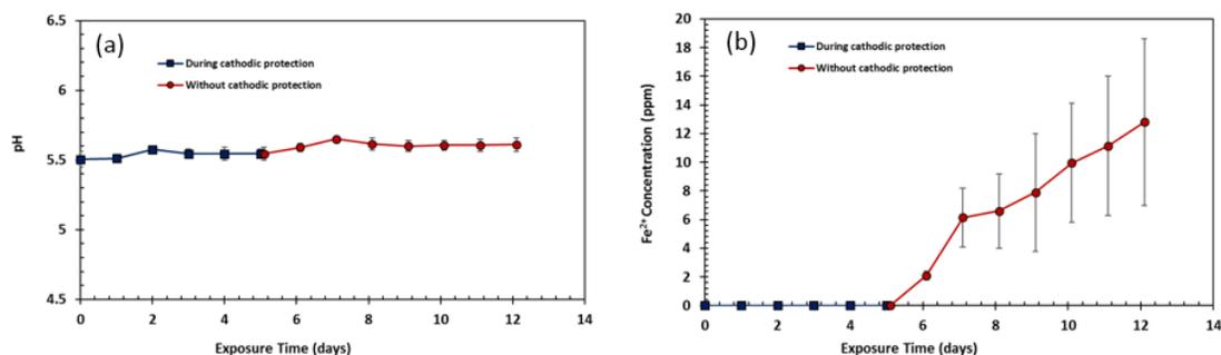
Figure 53. pH (a) and  $\text{Fe}^{2+}$  concentration (b) variation over time during and without cathodic protection ( $80^\circ\text{C}$ , bulk solution pH 5.5,  $\text{pCO}_2$  0.53 bar, 6000 ppm  $\text{Ca}^{2+}$ , 0.60 M ionic strength, and 20 rpm)
