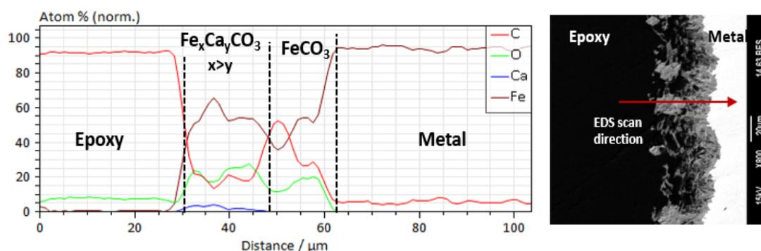
Figure 35. Elemental analysis (line scan) of cross-sectioned corrosion products formed on a specimen exposed to  $\text{CaCO}_3$ -saturated solution for 7 days at pH 6.2
