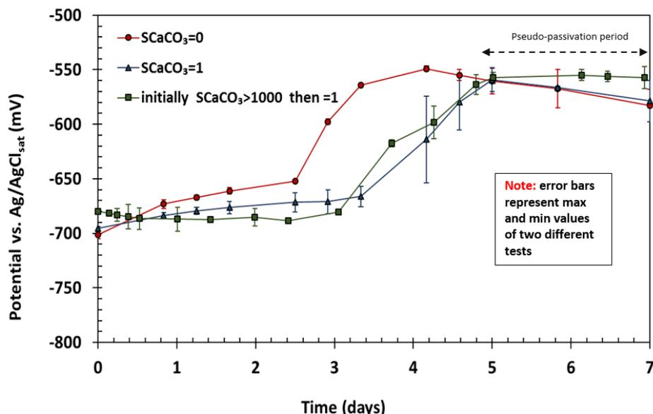
Figure 63. Comparison of OCP over time for UNS G10180 exposed to solutions with different  $CaCO_3$  saturation levels ( $80^\circ C$ ,  $pCO_2$  0.53 bar, 20 rpm, pH 6.2, ionic strength 0.18 M,  $[Ca^{2+}] \sim 160$  ppm)
