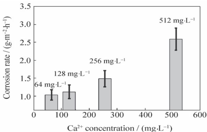
Figure 9. Corrosion rate *versus* different concentrations of  $\text{Ca}^{2+}$  for X65 specimens at  $75^\circ\text{C}$  and 10 bar  $\text{pCO}_2$  after 10 days of exposure (reproduced with permission [43])
