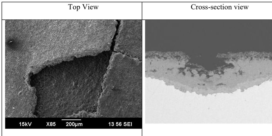
Figure 93. SEM images (top and cross section view) of ruptured corrosion products observed on specimens exposed to  $\text{MgCO}_3$ -saturated solution with 4,200 ppm  $\text{Mg}^{2+}$  at  $80^\circ\text{C}$ ,  $p\text{CO}_2$  0.53 bar, 0.58 m/s, pH 5.5, ionic strength 0.6 M, 1 wt.% NaCl
