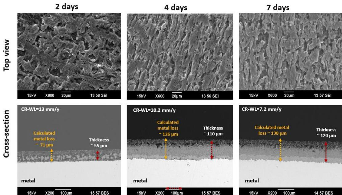
Figure 91. SEM images (top and cross-section view) of the development of surface layers over time for the experiment with presence of 4,200 ppm  $\text{Mg}^{2+}$  ( $S_{\text{MgCO}_3} = 1$ ) at  $80^\circ\text{C}$ ,  $\text{pCO}_2$  0.53 bar, 0.58 m/s, pH 5.5, ionic strength 0.6M, 1 wt.% NaCl
