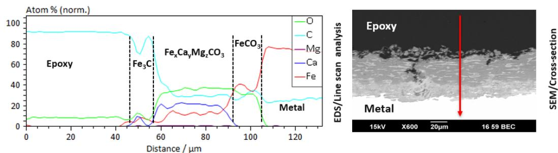
Figure 100. EDS line scan analysis of the surface layers developed on a specimen after 7 days of exposure to a  $\text{CaCO}_3$ -saturated electrolyte with 857 ppm  $\text{Mg}^{2+}$  at  $80^\circ\text{C}$ ,  $p\text{CO}_2$  0.53 bar, 0.58 m/s, pH 5.5, ionic strength 0.6M
