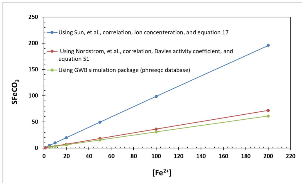
Figure 103. Effect of non-ideality: comparison of iron carbonate saturation ( $S_{\text{FeCO}_3}$ ) calculation using Equation 17, Equation 51, and GWB simulation package at 80°C,  $p\text{CO}_2$  0.53 bar, bulk solution pH 6.2, 0.18 M ionic strength
