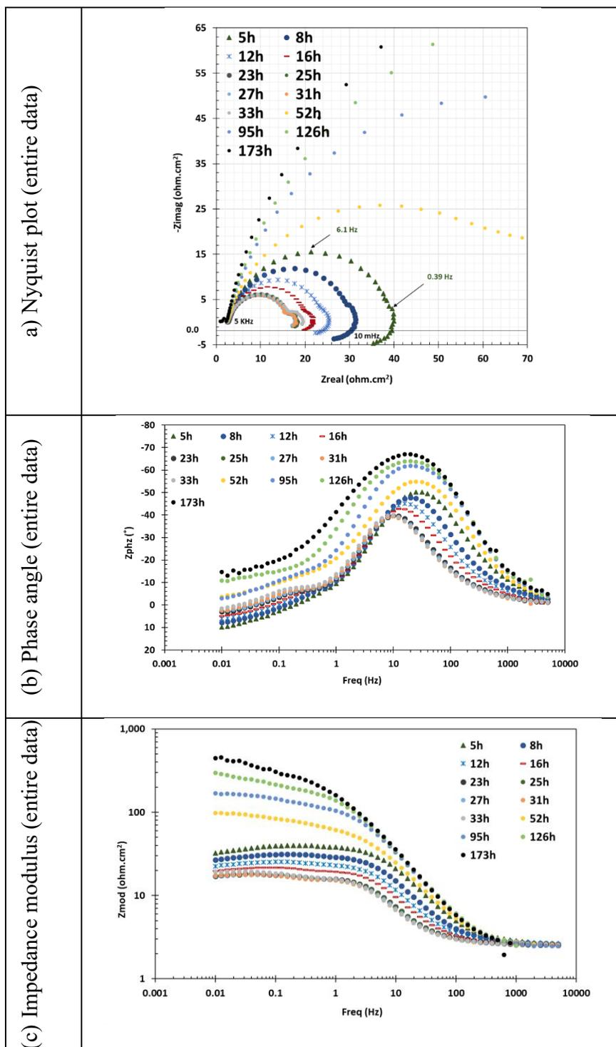
Figure 113. EIS spectra obtained over time from an experiment with presence of 6000 ppm  $\text{Ca}^{2+}$  ( $S_{\text{CaCO}_3} = 1$ ) conducted at  $80^\circ\text{C}$ ,  $p\text{CO}_2$  0.53 bar, bulk solution pH 5.5, 0.60 M ionic strength, and 20 rpm: Nyquist plot (a), phase angle (b), and Impedance modulus (c)
