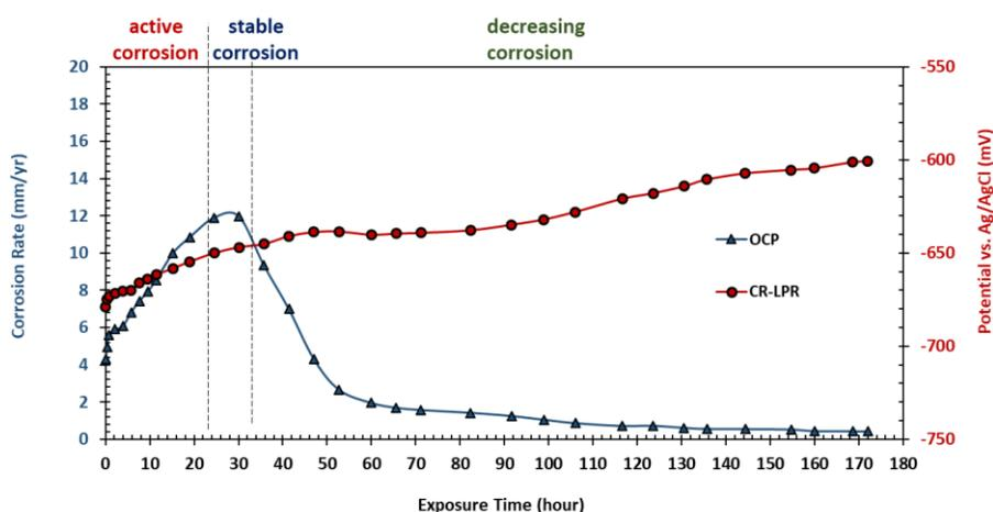
Figure 112. LPR corrosion rate and OCP variation over time for an experiment with presence of 6000 ppm  $\text{Ca}^{2+}$  ( $S_{\text{CaCO}_3} = 1$ ) conducted at  $80^\circ\text{C}$ ,  $\text{pCO}_2$  0.53 bar, bulk solution pH 5.5, 0.60 M ionic strength, and 20 rpm
