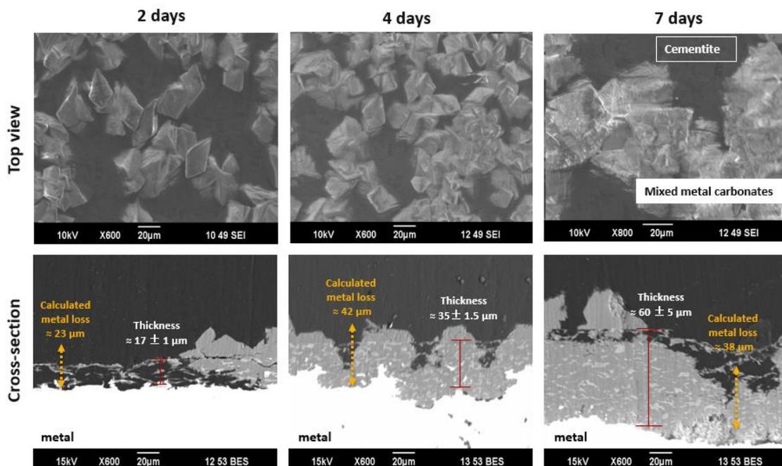
Figure 44. SEM images (top and cross-section view) of the development of surface layers over time for the experiments conducted in the presence of 6000 ppm  $\text{Ca}^{2+}$  ( $S_{\text{CaCO}_3} = 1$ ) at 80°C,  $\text{pCO}_2$  0.53 bar, bulk solution pH 5.5, 0.60 M ionic strength, and 20 rpm
