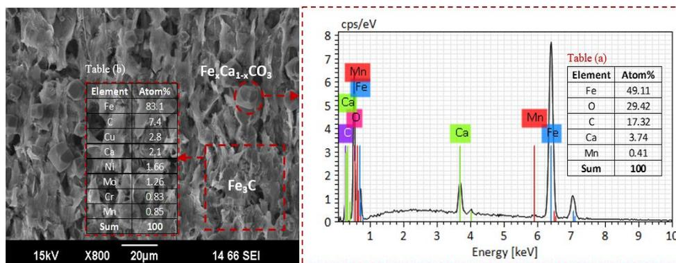
Figure 33. SEM/EDS analysis (top view) of the surface layers on UNS G10180 developed from a solution saturated with  $\text{CaCO}_3$  after 7 days of exposure at pH 6.2
