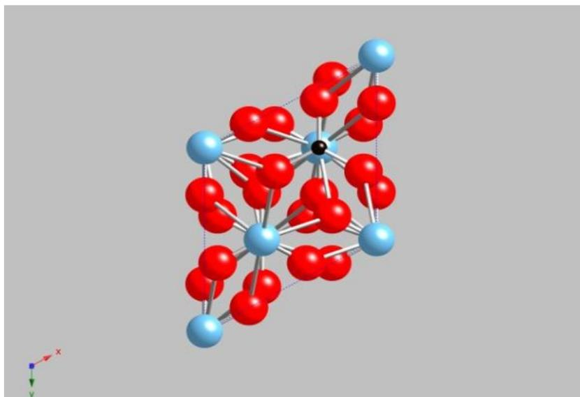
Figure 4. Hexagonal single unit cell of calcite ( $\text{CaCO}_3$ ; blue = Ca, red = O, black =C)
