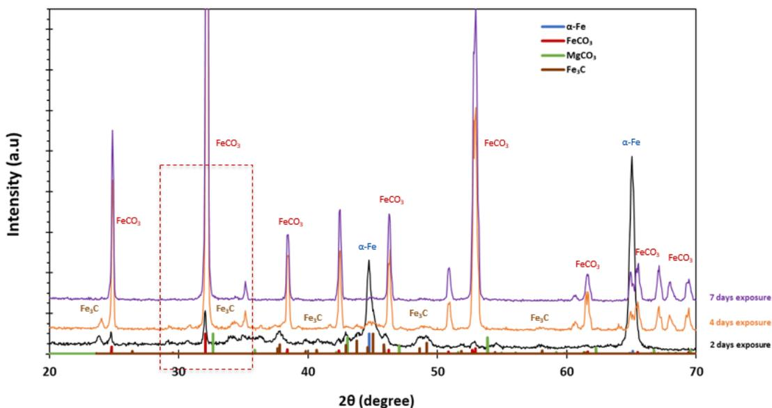
Figure 85. XRD patterns of surface layers detected on the steel surface after 2, 4, and 7 days of exposure to an electrolyte saturated with  $\text{MgCO}_3$  at  $80^\circ\text{C}$ ,  $p\text{CO}_2$  0.53 bar, 100 ppm  $\text{Mg}^{2+}$ , 0.58 m/s, pH 6.2, ionic strength 0.18 M, 1wt% NaCl
