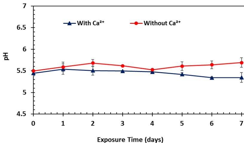
Figure 36. Variation of bulk solution pH over time for experiments with and without 6000 ppm  $\text{Ca}^{2+}$  ( $S_{\text{CaCO}_3} = 1$ ) at  $80^\circ\text{C}$ ,  $\text{pCO}_2$  0.53 bar, 0.60 M ionic strength, and 20 rpm
