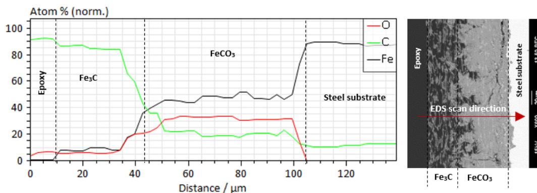
Figure 43. EDS line scan analysis of the surface layers developed after 7 after 7 days of exposure to the experiment without  $\text{Ca}^{2+}$  at  $80^\circ\text{C}$ ,  $\text{pCO}_2$  0.53 bar, bulk solution pH 5.5, 0.60 M ionic strength, and 20 rpm
