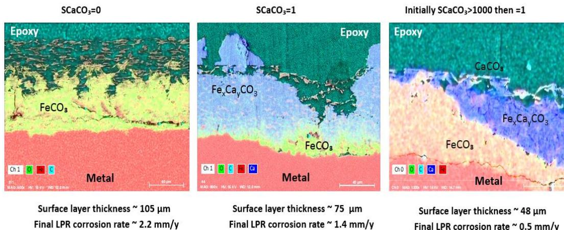
Figure 77. EDS mapping analysis of the cross-sectioned surface layers after 7 days of exposure to different  $\text{CaCO}_3$  saturation levels at  $80^\circ\text{C}$ ,  $p\text{CO}_2$  0.53 bar, 0.58 m/s, pH 5.5, ionic strength 0.6 M,  $[\text{Ca}^{2+}] \sim 6000$  ppm
