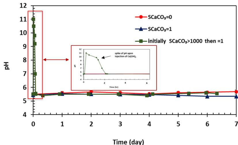
Figure 69. Variation of bulk solution pH over time for the experiments with different  $CaCO_3$  saturation levels ( $80^\circ C$ ,  $pCO_2$  0.53 bar, 20 rpm, pH 5.5, ionic strength 0.6 M,  $[Ca^{2+}] \sim 6000$  ppm)
