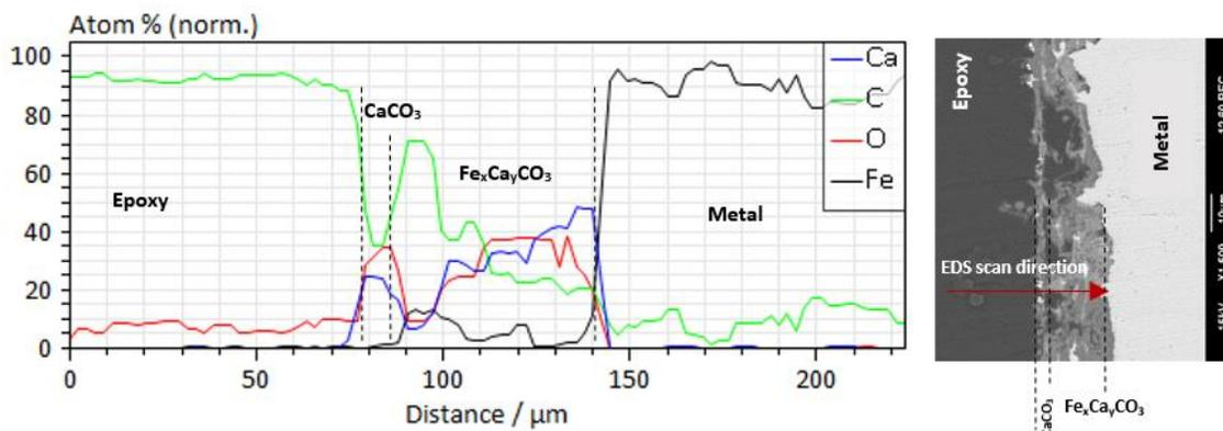
Figure 56. Chemical composition of the layers at the steel surface after 7 days of exposure to a  $\text{CaCO}_3$ -saturated solution without cathodic protection of specimen at pH 5.5,  $80^\circ\text{C}$ , 0.53 bar  $\text{pCO}_2$ , ionic strength 0.6M, 6000 ppm  $\text{Ca}^{2+}$ , 20 rpm
