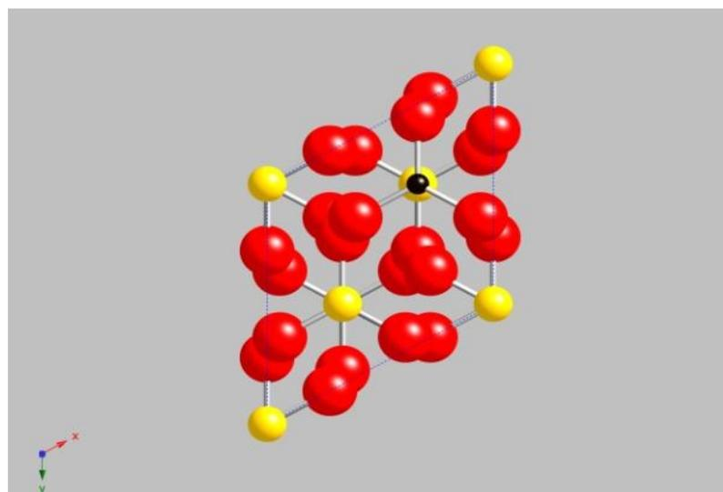
Figure 5. Hexagonal single unit cell of magnesite ( $\text{MgCO}_3$ ; yellow = Mg, red = O, black =C)
