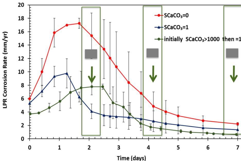
Figure 71. Comparison of LPR corrosion behavior of UNS G10180 exposed to solutions with different  $CaCO_3$  saturation level at  $80^\circ C$ ,  $pCO_2$  0.53 bar, 0.58 m/s, pH 5.5, ionic strength 0.6 M,  $[Ca^{2+}] \sim 6000$  ppm
