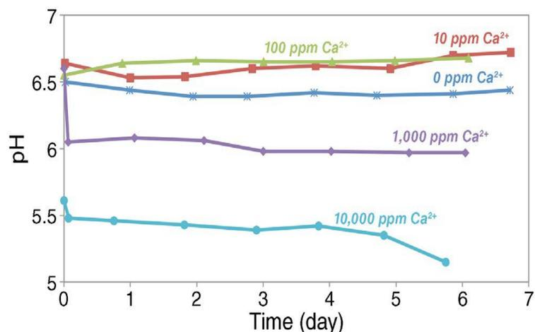
Figure 12. Variation of pH over time for different concentrations of Ca<sup>2+</sup> at 80°C, pCO<sub>2</sub> 0.53 bar, 1wt. % NaCl, and 10 ppm Fe<sup>2+</sup> (note the difference in the electrolytes' pH caused by precipitation of CaCO<sub>3</sub> in high concentration of calcium ions). reproduced with permission [44]
