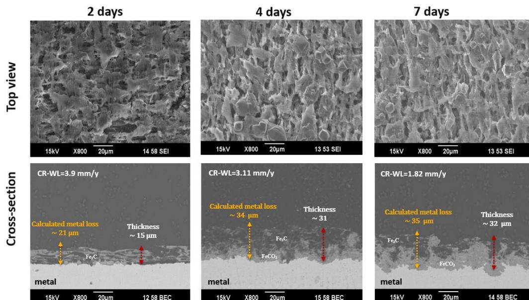
Figure 23. SEM images of top view and cross-sectional morphology of surface layers exposed to solution in the absence of  $\text{CaCO}_3$  at pH 6.2 (note: the CR-WL provided here is specific for the experiment in which the surface characterization is presented here)
