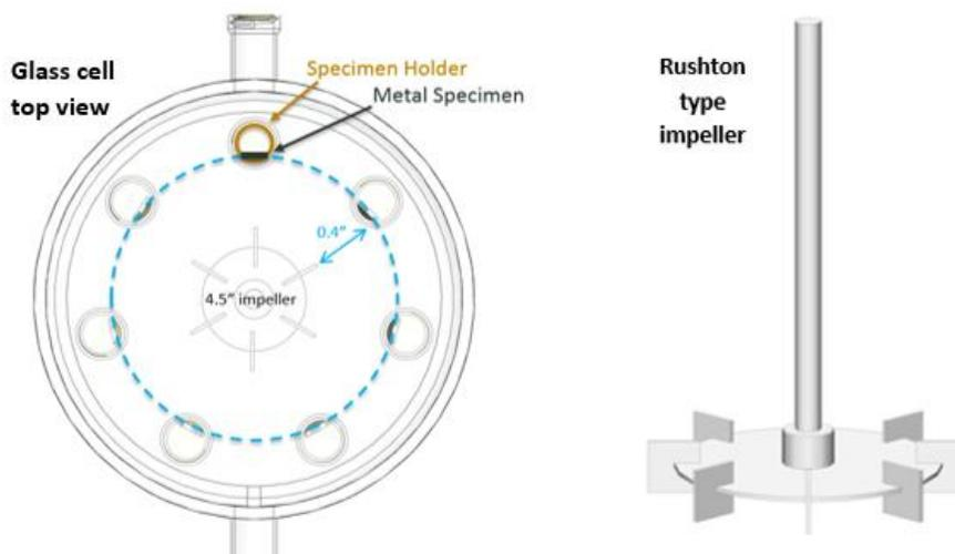
Figure 15. Schematic view of the system equipped with impeller and  $[\text{Fe}^{2+}]/[\text{H}^+]$  control loops. The impeller diameter was 4.5", the distance between the impeller blades and the specimen surface was 0.4", and the glass cell had an 8" internal diameter. (All drawings courtesy of Cody Shafer, ICMT, OU.)
