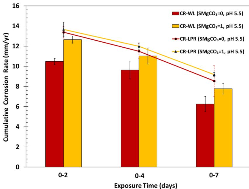
Figure 88. Cumulative corrosion rate by WL (bar chart) and LPR (line chart) techniques over time for solution with and without 4,200 ppm Mg<sup>2+</sup> (80°C, pCO<sub>2</sub> 0.53 bar, 0.58 m/s, pH 5.5, ionic strength 0.6 M, 1 wt.% NaCl)
