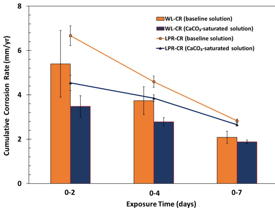
Figure 30. Comparison of cumulative corrosion rate obtained by LPR and WL methods with and without CaCO<sub>3</sub> after 2, 4, and 7 days of exposure at pH 6.2
