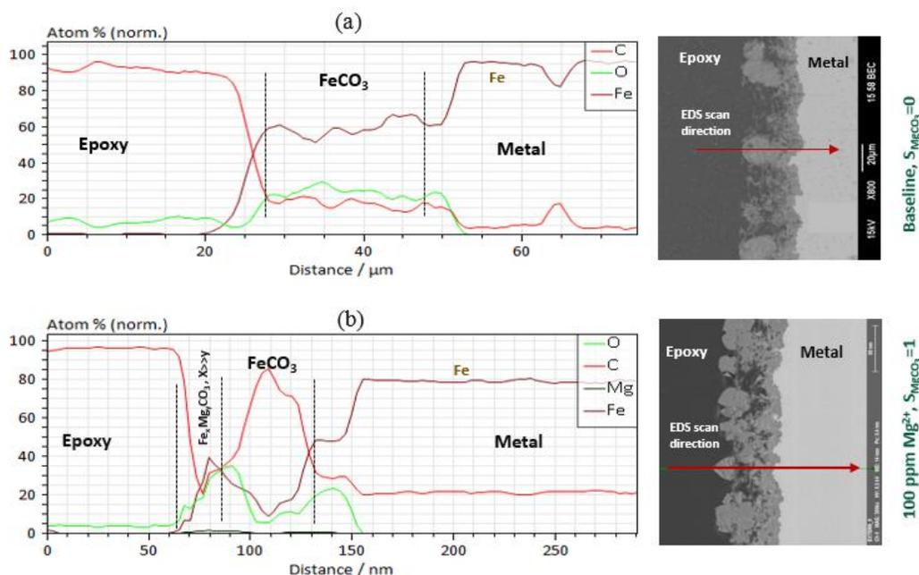
Figure 84. EDS line scan analysis of the surface layers developed on the specimens after 7 days of exposure to electrolytes without (a) and with (b) 100 ppm  $Mg^{2+}$  at 80°C,  $pCO_2$  0.53 bar, 0.58 m/s, pH 6.2, ionic strength 0.18 M, 1wt% NaCl
