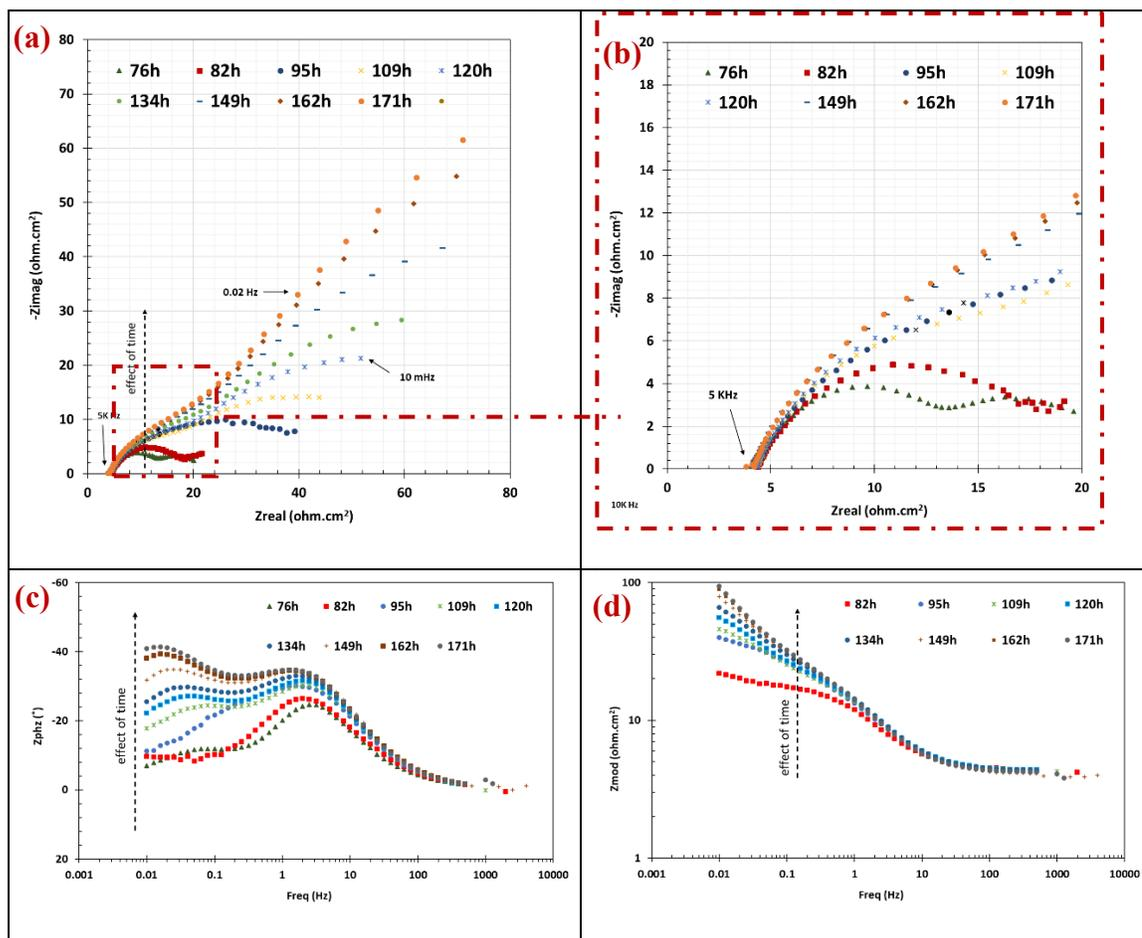
Figure 111. EIS results obtained from decreasing corrosion period of a baseline experiment ( $S_{CaCO_3} = 0$ ) conducted at  $80^\circ\text{C}$ ,  $p\text{CO}_2$  0.53 bar, bulk solution pH 5.5, 0.60 M ionic strength, and 20 rpm: (a) and (b) Nyquist plots, (c) phase angle, and (d) impedance modulus
