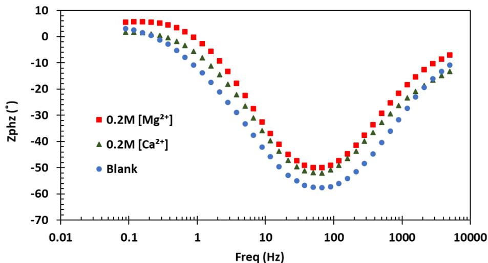
Figure 118. Phase angle diagrams obtained from a blank,  $\text{Ca}^{2+}$ -containing, and  $\text{Mg}^{2+}$ -containing solution at  $40^\circ\text{C}$ ,  $\text{pCO}_2$  0.93 bar, bulk solution pH 4.64, 0.77 M ionic strength, and 1500 rpm
