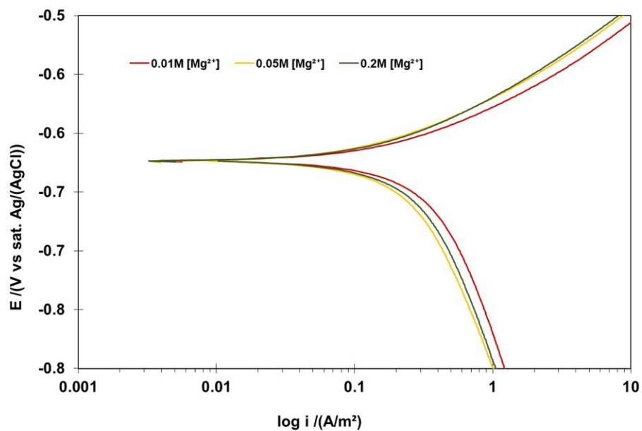
Figure 122. Cathodic polarization of mild steel in presence of different concentration of  $\text{Mg}^{2+}$  (0.01, 0.05, and 0.2 M) at 1°C,  $p\text{CO}_2$  0.99 bar, bulk solution pH 4.23, ionic strength 0.2M to 0.77M, and 2000 rpm
