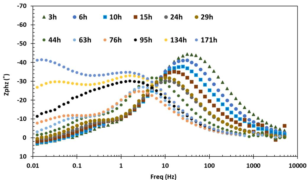
Figure 107. Phase angle. EIS spectra obtained over time from a baseline experiment ( $S_{CaCO_3} = 0$ ) conducted at 80°C,  $pCO_2$  0.53 bar, bulk solution pH 5.5, 0.60 M ionic strength, and 20 rpm
