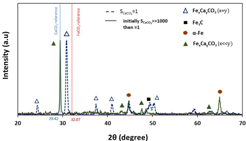
Figure 78. X-ray diffraction patterns of surface layers detected on the steel surface after 7 days of exposure to electrolytes with  $S_{\text{CaCO}_3} = 1$  and initially  $S_{\text{CaCO}_3} \gg 1000$  at  $80^\circ\text{C}$ ,  $\text{pCO}_2$  0.53 bar, 20 rpm, pH 5.5, ionic strength 0.6 M,  $[\text{Ca}^{2+}] \sim 6000$  ppm.
