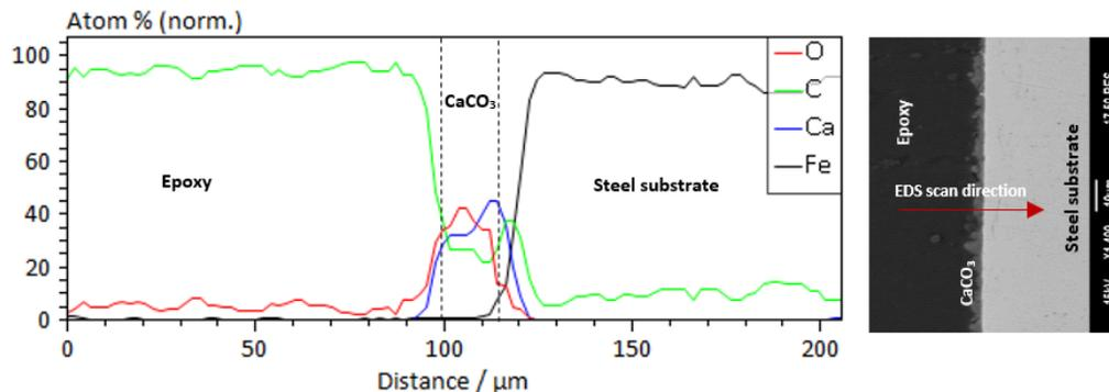
Figure 51. EDS line scan results showing distribution of Ca, C, O, and Fe within the surface layers; formation of  $\text{CaCO}_3$  scale ( $80^\circ\text{C}$ , bulk solution pH 5.5,  $p\text{CO}_2$  0.53 bar, 6000 ppm  $\text{Ca}^{2+}$ , 0.60 M ionic strength, and 20 rpm)
