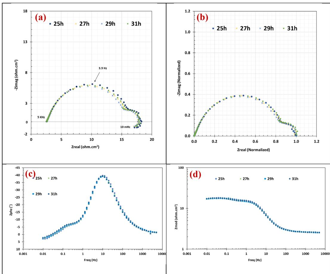
Figure 115. EIS results obtained from stable corrosion period of an experiment with presence of 6000 ppm  $\text{Ca}^{2+}$  ( $S_{\text{CaCO}_3} = 1$ ) conducted at 80°C,  $\text{pCO}_2$  0.53 bar, bulk solution pH 5.5, 0.60 M ionic strength, and 20 rpm: (a) Nyquist plots (b) normalized Nyquist plots (c) phase angle, and (d) impedance modulus
