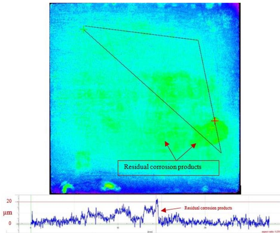
Figure 86. Example of profilometry of the specimen after removing the corrosion products (7 days of exposure to solution saturated with  $\text{MgCO}_3$  at pH 6.2,  $80^\circ\text{C}$ ,  $\text{pCO}_2$  0.53 bar, 100 ppm  $\text{Mg}^{2+}$ , ionic strength 0.18 M, 1 wt.% NaCl, 100 ppm  $\text{Mg}^{2+}$ )
