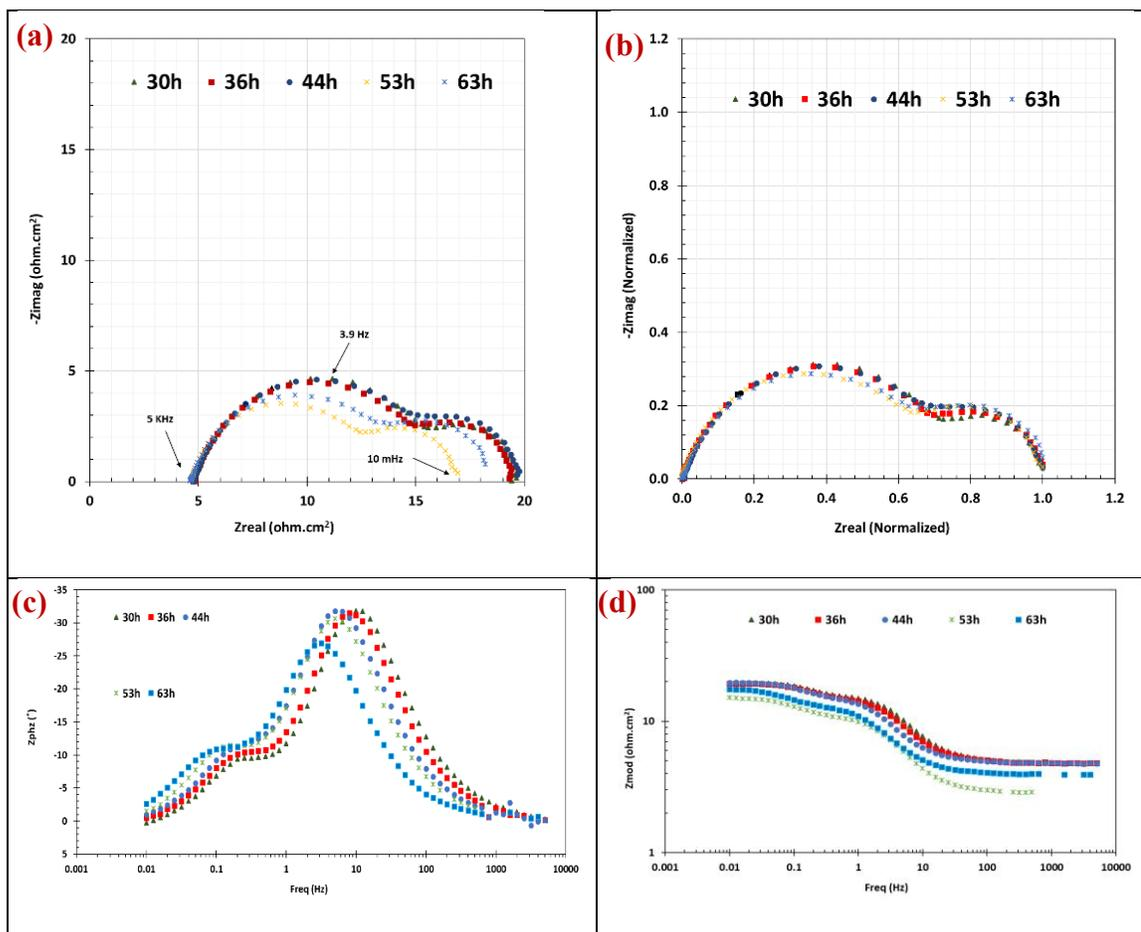
Figure 110. EIS results obtained from stable corrosion period of a baseline experiment ( $S_{CaCO_3} = 0$ ) conducted at  $80^\circ\text{C}$ ,  $p\text{CO}_2$  0.53 bar, bulk solution pH 5.5, 0.60 M ionic strength, and 20 rpm: (a) Nyquist plots (b) normalized Nyquist plots (c) phase angle, and (d) impedance modulus
