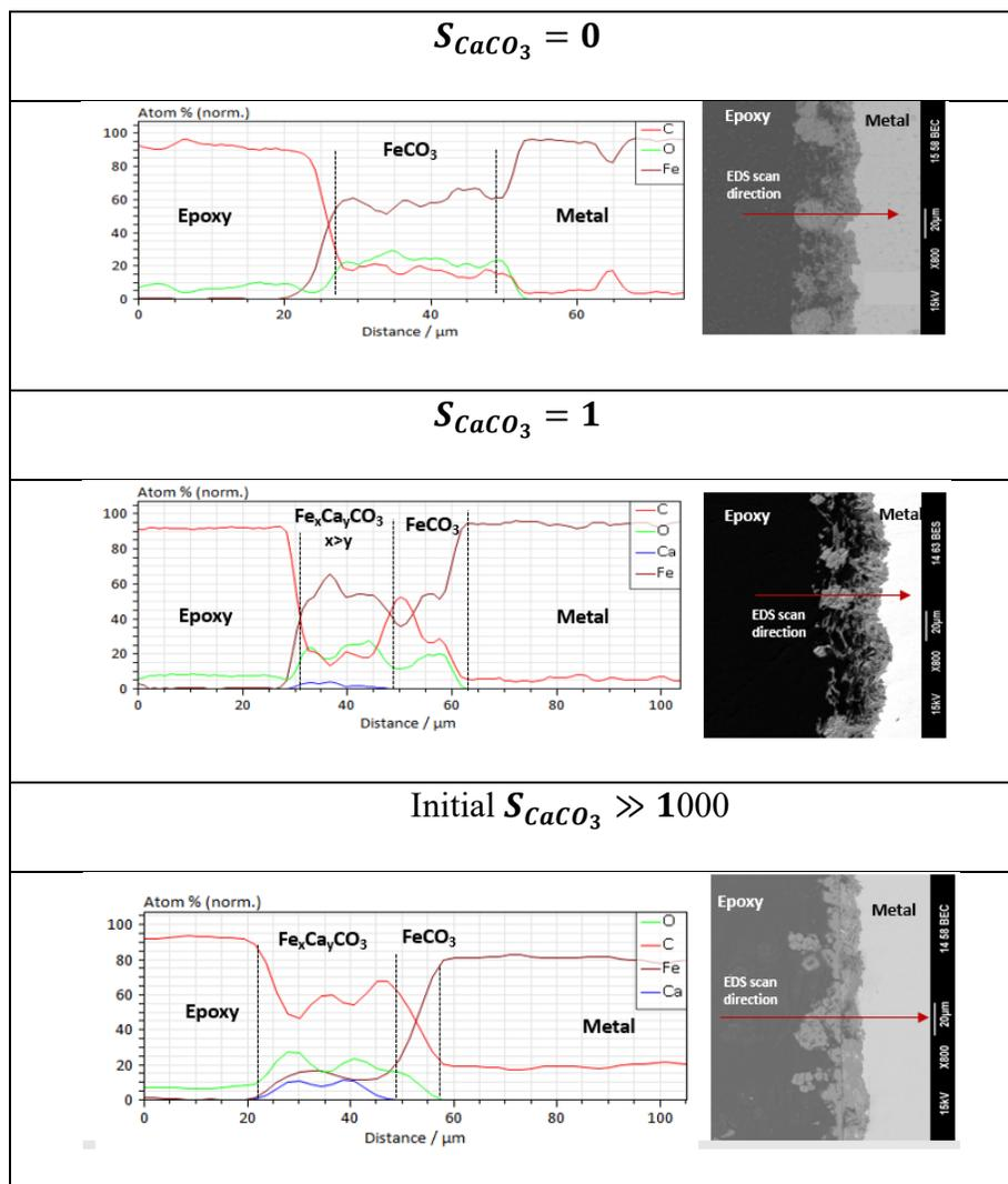
Figure 66. EDS line scan analysis of the surface layers developed on the specimens after 7 days of exposure to electrolytes with different  $\text{CaCO}_3$  saturation level at  $80^\circ\text{C}$ ,  $\text{pCO}_2$  0.53 bar, 0.58 m/s, pH 6.2, ionic strength 0.18 M,  $[\text{Ca}^{2+}] \sim 160$  ppm
