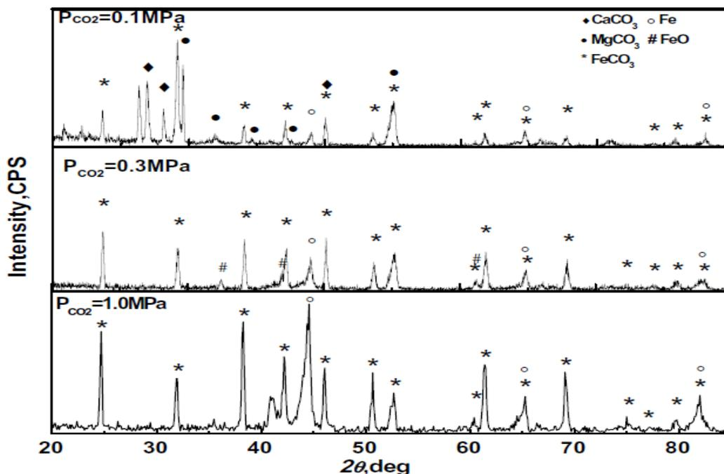
Figure 7. XRD patterns of the layers formed on X65 carbon steel specimens at various  $p_{\text{CO}_2}$  values, quiescent condition,  $65^\circ\text{C}$ ,  $64 \text{ ppm Ca}^{2+}$ , and  $72 \text{ ppm Mg}^{2+}$  (reproduced with permission [46])
