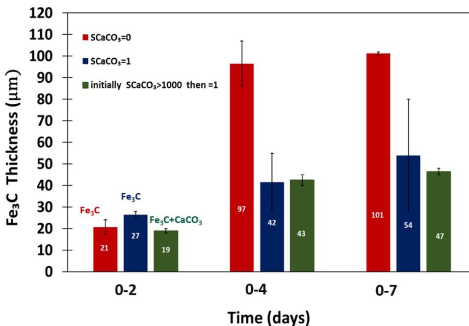
Figure 75.  $Fe_3C$  growth on mild steel over time exposed to solutions with different  $CaCO_3$  saturation levels at 80°C,  $pCO_2$  0.53 bar, 20 rpm, pH 5.5, ionic strength 0.6 M,  $[Ca^{2+}] \sim 6000$  ppm
