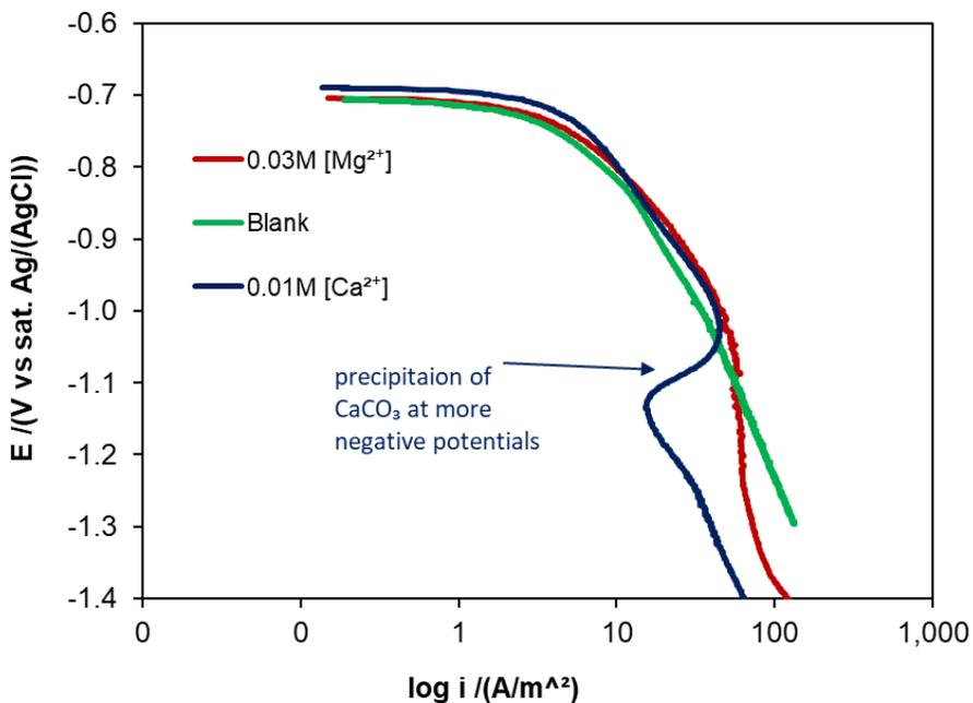
Figure 121. Cathodic polarization of mild steel in presence of a blank, Ca<sup>2+</sup>-containing, and Mg<sup>2+</sup>-containing solution at 80°C, pCO<sub>2</sub> 0.53 bar, bulk solution pH 6.2, and 250 rpm
