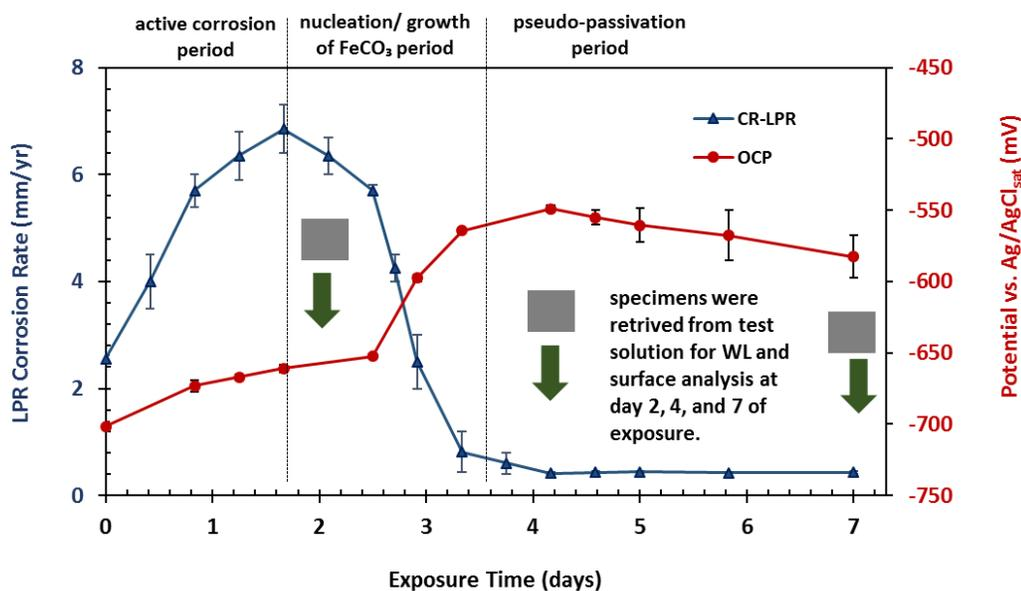
Figure 21. Change in LPR corrosion rate and open circuit potential with time explained by three different periods: active corrosion, nucleation/growth of  $\text{FeCO}_3$ , and pseudo-passivation (UNS G10180, 80 °C,  $p\text{CO}_2$  0.53 bar, pH 6.2, NaCl 1wt%,  $4 < S_{\text{FeCO}_3} < 14$ ,  $S_{\text{CaCO}_3} = 0$ , velocity 0.58 m/s)
