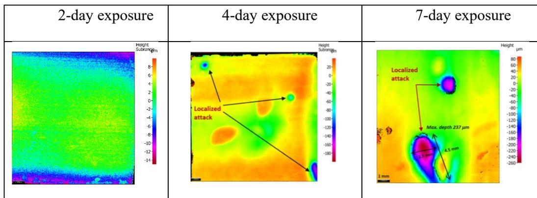
Figure 94. Profilometry of specimens after removing of corrosion product layers ( $\text{MgCO}_3$ -saturated solution with 4,200 ppm  $\text{Mg}^{2+}$  at  $80^\circ\text{C}$ ,  $\text{pCO}_2$  0.53 bar, 0.58 m/s, pH 5.5, ionic strength 0.6M, 1 wt.% NaCl)
