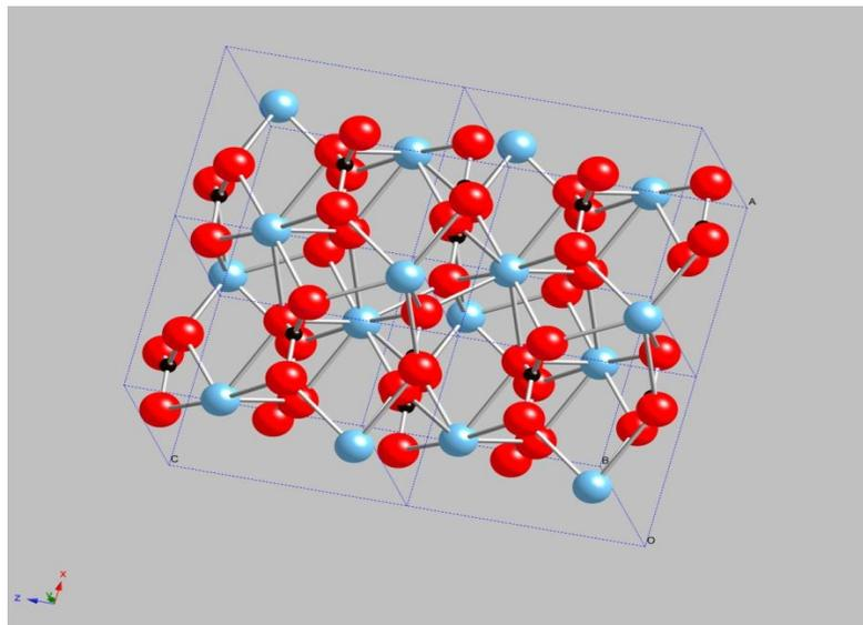
Figure 6. Orthorhombic crystal structure of aragonite ( $\text{CaCO}_3$ ; blue = Ca, red = O, black =C), four unit cells
