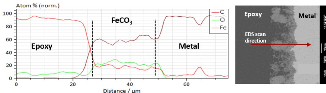
Figure 25. EDS analysis (line scan) of cross-sectioned corrosion products formed on a specimen exposed to the baseline solution for 7 days at pH 6.2
