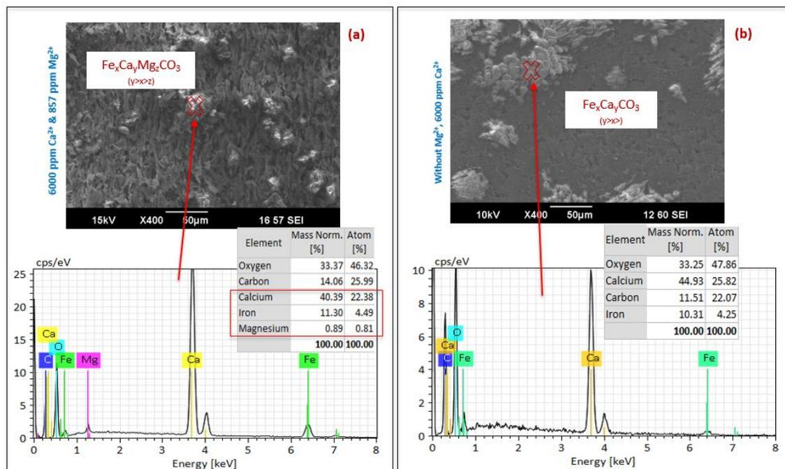
Figure 99. Comparison of SEM/EDS results for two solutions at 80°C,  $\text{pCO}_2$  0.53 bar, 0.58 m/s, pH 5.5, ionic strength 0.68 M [(a);  $\text{Ca}^{2+}/\text{Mg}^{2+}=7$ ,  $\text{SCaCO}_3=1$  and (b)  $\text{Ca}^{2+}=6000$  ppm,  $\text{SCaCO}_3=1$ ]
