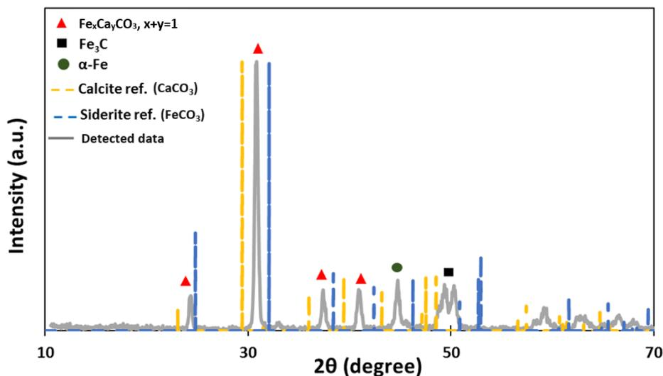
Figure 47. XRD pattern of the surface layers formed on UNS G10180 specimen after 7 days of exposure to a  $\text{CaCO}_3$ -saturated solution (6000 ppm  $\text{Ca}^{2+}$ ) at  $80^\circ\text{C}$ , bulk solution pH 5.5,  $p\text{CO}_2$  0.53 bar, 0.60 M ionic strength, and 20 rpm
