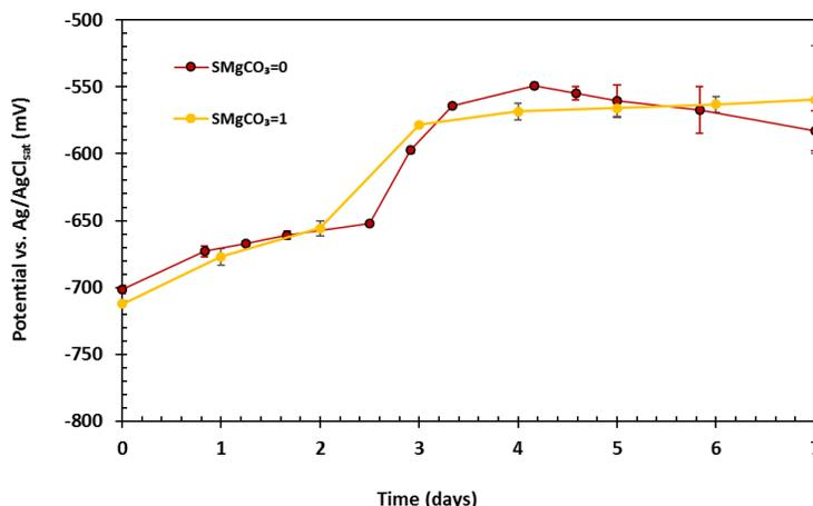
Figure 82. Comparison of OCP over time for UNS G10180 exposed to solutions with and without 100 ppm  $Mg^{2+}$  ( $80^{\circ}C$ ,  $pCO_2$  0.53 bar, 0.58 m/s, pH 6.2, ionic strength 0.18 M, 1 wt.% NaCl)
