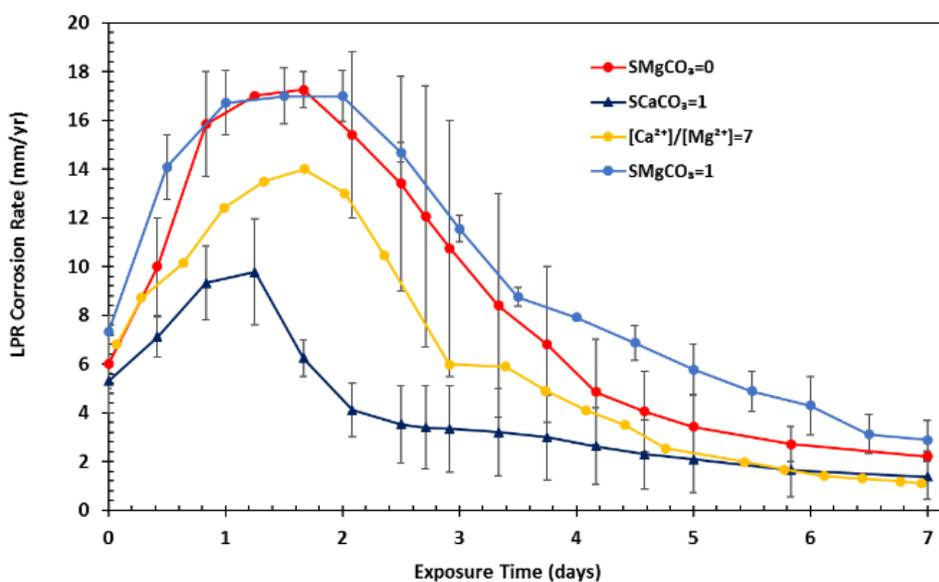
Figure 96. Trend of corrosion rate obtained by LPR over time at 80°C,  $\text{pCO}_2$  0.53 bar, 0.58 m/s, pH 5.5, ionic strength 0.6M [baseline (red), 6000 ppm  $\text{Ca}^{2+}$  (dark blue),  $\text{Ca}^{2+}/\text{Mg}^{2+}=7$  (yellow), and 4200 ppm  $\text{Mg}^{2+}$  (light blue)]
