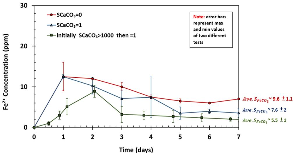
Figure 60. Variation of  $[\text{Fe}^{2+}]$  over time for the experiments with different  $\text{CaCO}_3$  saturation levels ( $80^\circ\text{C}$ ,  $p\text{CO}_2$  0.53 bar, 20 rpm, pH 6.2, ionic strength 0.18 M,  $[\text{Ca}^{2+}] \sim 160$  ppm)
