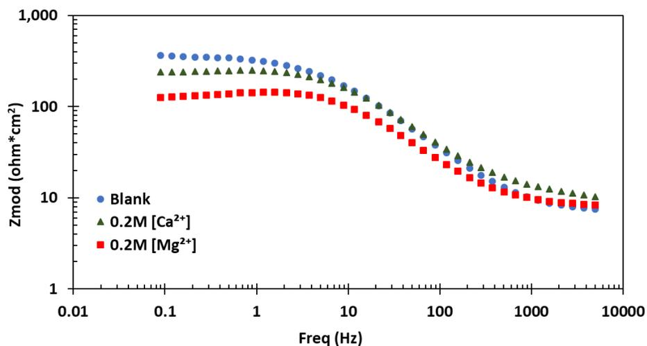
Figure 119. Impedance modulus diagrams obtained from a blank,  $\text{Ca}^{2+}$ -containing, and  $\text{Mg}^{2+}$ -containing solution at  $40^\circ\text{C}$ ,  $\text{pCO}_2$  0.93 bar, bulk solution pH 4.64, 0.77 M ionic strength, and 1500 rpm
