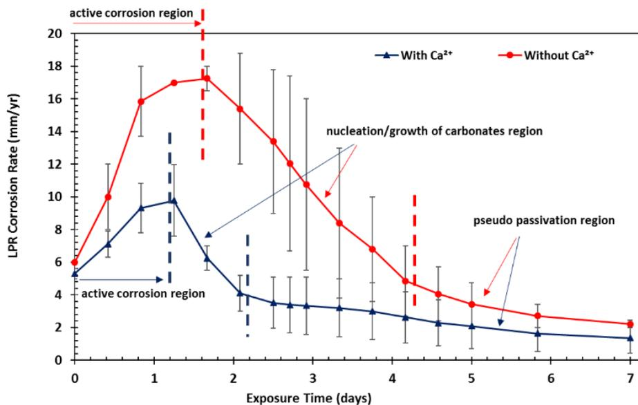
Figure 38. Comparison of LPR corrosion rates of UNS G10180 exposed to solutions without and with 6000 ppm  $\text{Ca}^{2+}$  ( $S_{\text{CaCO}_3} = 1$ ) at 80°C,  $p\text{CO}_2$  0.53 bar, bulk solution pH 5.5, 0.60 M ionic strength, and 20 rpm
