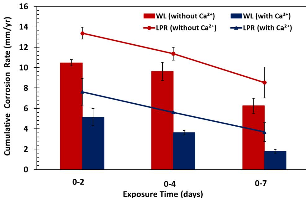
Figure 39. WL and LPR cumulative corrosion rate over time for solutions without and with 6000 ppm Ca<sup>2+</sup> ( $S_{CaCO_3} = 1$ ) at 80°C, pCO<sub>2</sub> 0.53 bar, bulk solution pH 5.5, 0.60 M ionic strength, and 20 rpm
