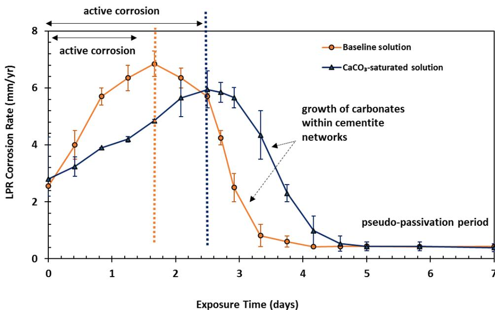
Figure 29. Comparison of LPR corrosion behavior of UNS G10180 exposed to CaCO<sub>3</sub>-saturated and baseline (CaCO<sub>3</sub>-free) aqueous conditions at pH 6.2
