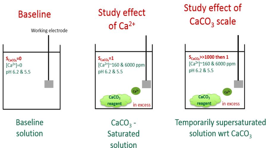
Figure 58. Schematic of experimental design of three different  $\text{CaCO}_3$  saturation levels in various solution pH and  $[\text{Ca}^{2+}]$  at  $80^\circ\text{C}$ ,  $p\text{CO}_2$  0.53 bar, 1wt% NaCl, and 20 rpm
