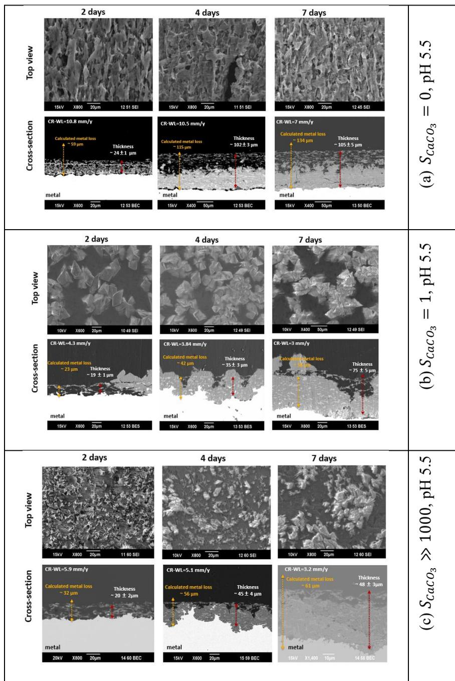
Figure 74. SEM images (top and cross-section view) of the development of surface layers over time for the experiment with different  $CaCO_3$ -saturation level at  $80^\circ C$ ,  $pCO_2$  0.53 bar, 20 rpm, pH 5.5, ionic strength 0.6 M
