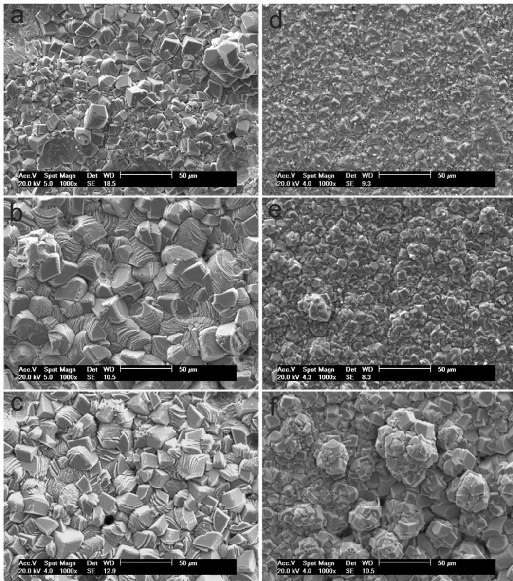
Figure 13. SEM images of surface layers' morphology formed on low carbon steel after 72, 336, 672 hours of exposure in CO<sub>2</sub>-saturated solutions (a, b, and c) without and (d, e, and f) with CaCO<sub>3</sub> (reproduced with permission [50])
