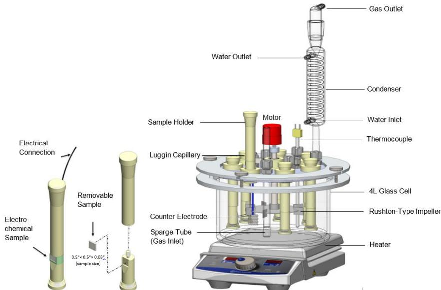
Figure 16. Schematic view of removeable specimen holder, electrochemical sample configuration, and the experimental setup.
