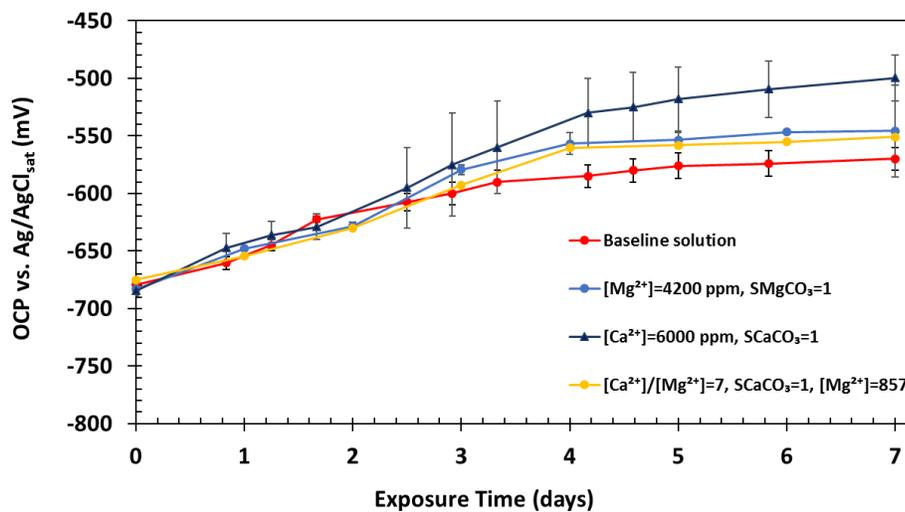
Figure 98. Comparison of OCP over time for UNS G10180 exposed to various solutions at 80°C, pCO<sub>2</sub> 0.53 bar, 0.58 m/s, pH 5.5, ionic strength 0.68 M [baseline (red), 6000 ppm Ca<sup>2+</sup> (dark blue), Ca<sup>2+</sup>/Mg<sup>2+</sup>=7 (yellow), and 4200 ppm Mg<sup>2+</sup> (light blue)]
