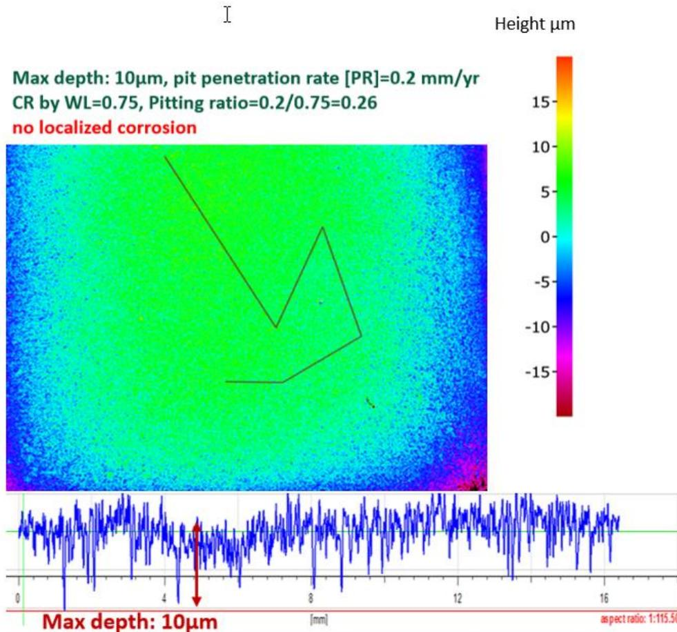
Figure 68. Example of profilometry of the specimen after removing the surface layer (7 days of exposure, initially  $\text{CaCO}_3$  supersaturated solution at pH 6.2,  $80^\circ\text{C}$ ,  $p\text{CO}_2$  0.53 bar, 20 rpm, and ionic strength 0.18 M)
