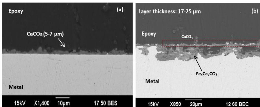
Figure 55. Comparison of surface layers morphology and thickness at the end of the polarization period (5 days exposure) and after exposure to the corrosive medium without cathodic protection (7 days exposure) at 80°C, bulk solution pH 5.5,  $\text{pCO}_2$  0.53 bar, 6000 ppm  $\text{Ca}^{2+}$ , 0.60 M ionic strength, and 20 rpm
