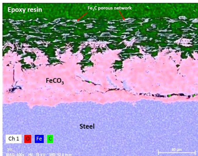
Figure 42. Cross-section SEM/EDS analysis of the corrosion products after 7 days of exposure to the experiment without  $\text{Ca}^{2+}$  at  $80^\circ\text{C}$ ,  $\text{pCO}_2$  0.53 bar, bulk solution pH 5.5, 0.60 M ionic strength, and 20 rpm
