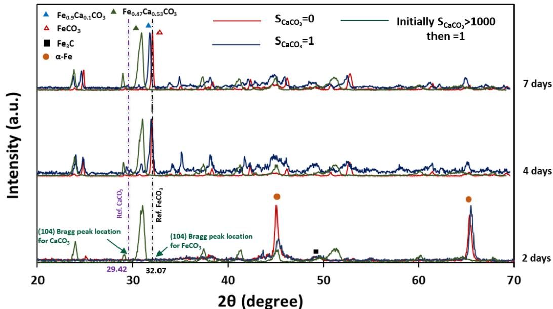
Figure 67. XRD patterns of surface layers detected on the steel surface after 2, 4, and 7 days of exposure to electrolytes with different  $\text{CaCO}_3$  saturation level at  $80^\circ\text{C}$ ,  $p\text{CO}_2$  0.53 bar, 0.58 m/s, pH 6.2, ionic strength 0.18 M,  $[\text{Ca}^{2+}] \sim 160$  ppm
