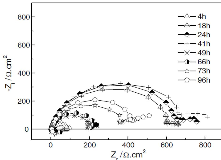
Figure 8. Nyquist plots *versus* time for API CT5 N80 materials in 3 wt.% NaCl + 1.5 wt.% CaCl<sub>2</sub> electrolyte at 57°C (reproduced with permission [47])
