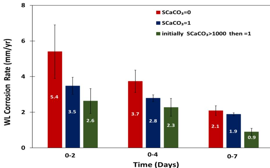
Figure 62. Cumulative corrosion rate by weight loss techniques over time for solution with different  $CaCO_3$  saturation levels (80°C,  $pCO_2$  0.53 bar, 20 rpm, pH 6.2, ionic strength 0.18 M,  $[Ca^{2+}] \sim 160$  ppm)
