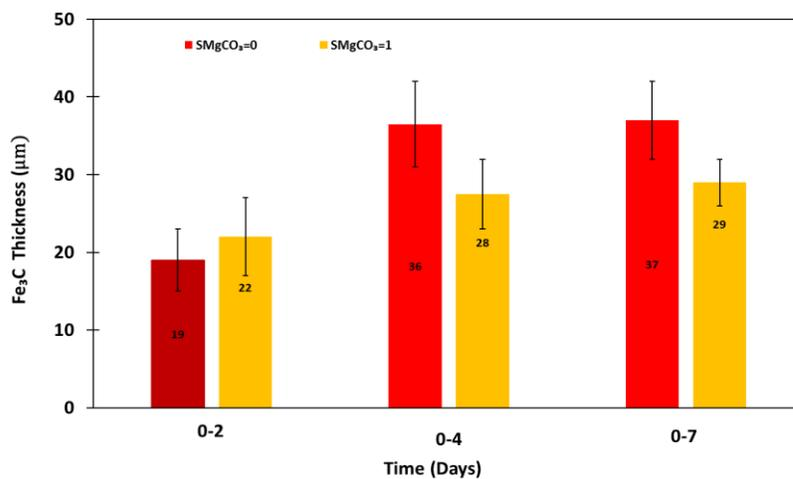
Figure 81. Evolution of Fe<sub>3</sub>C over time with and without presence of 100 ppm Mg<sup>2+</sup> (80°C, pCO<sub>2</sub> 0.53 bar, 0.58 m/s, pH 6.2, ionic strength 0.18 M, 1 wt.% NaCl)
