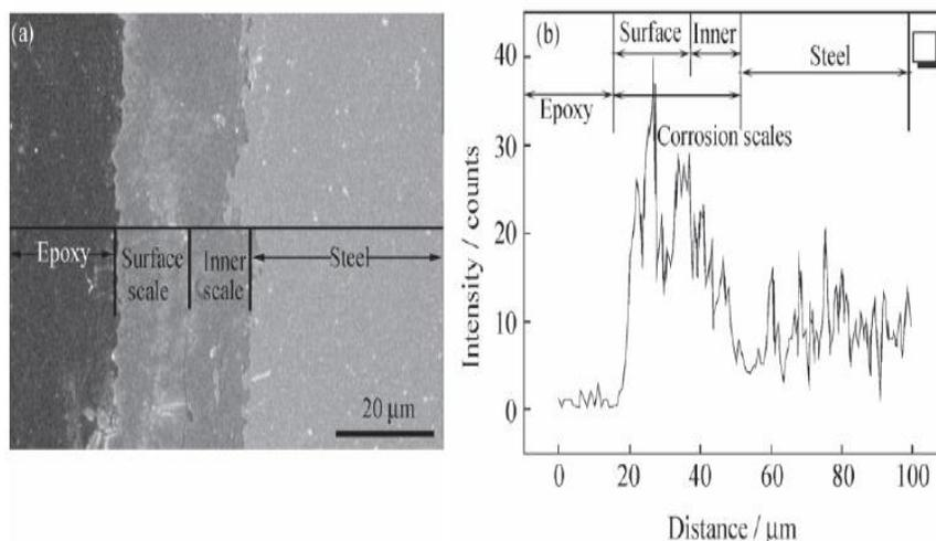
Figure 10. Elemental analysis for calcium in the bilayers formed on the steel surface. Note the higher concentration of calcium in the outer layer (“surface scale”) compared to the inner layer (“inner scale”) when the test solution contained 512 ppm  $\text{Ca}^{2+}$  (reproduced with permission [43])
