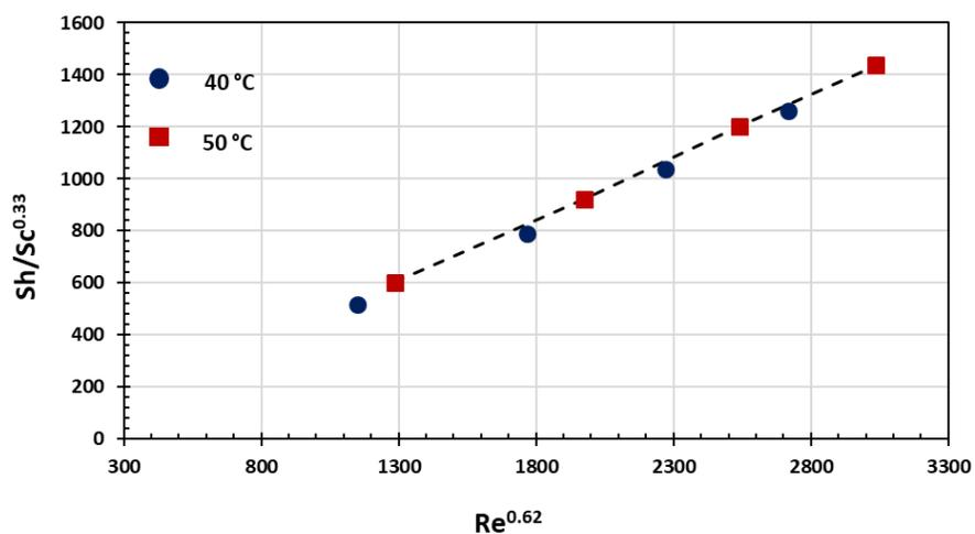
Figure 18. A straight-line fit of the mass transfer correlation developed for the experimental setup with impeller based on the relation between Sherwood (Sh), Reynolds (Re), and Schmidt (Sc) numbers
