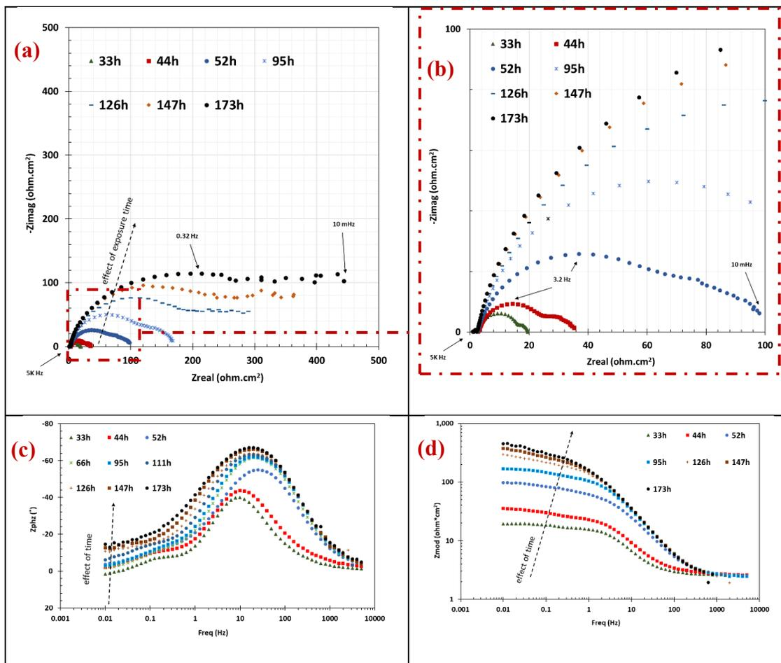
Figure 116. EIS results obtained from decreasing corrosion period of an experiment with presence of 6000 ppm  $\text{Ca}^{2+}$  ( $S_{\text{CaCO}_3} = 1$ ) conducted at 80°C,  $p\text{CO}_2$  0.53 bar, bulk solution pH 5.5, 0.60 M ionic strength, and 20 rpm: (a) and (b) Nyquist plots, (c) phase angle, and (d) impedance modulus
