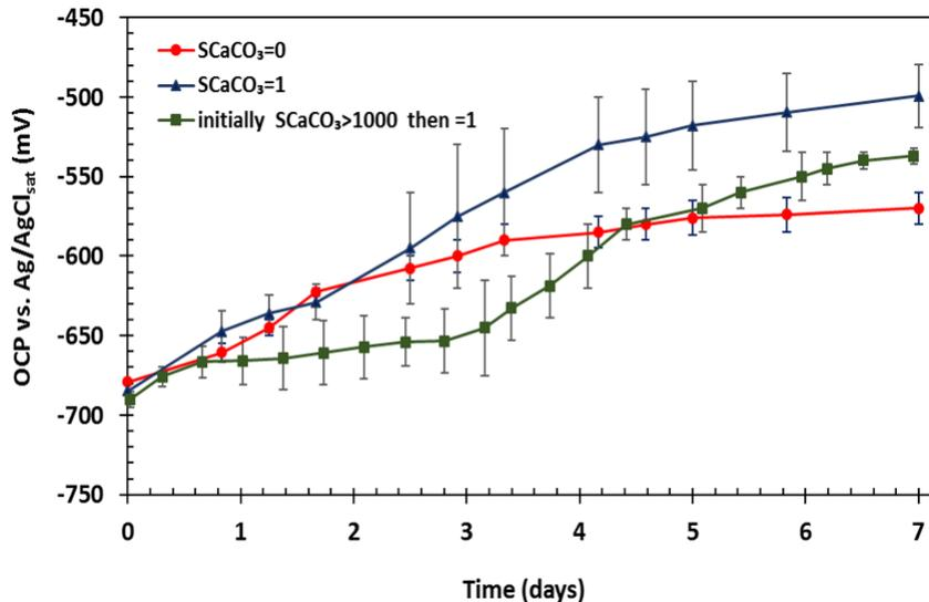
Figure 73. Comparison of OCP over time for UNS G10180 exposed to solutions with different  $\text{CaCO}_3$  saturation level at  $80^\circ\text{C}$ ,  $\text{pCO}_2$  0.53 bar, 20 rpm, pH 5.5, ionic strength 0.6 M,  $[\text{Ca}^{2+}] \sim 6000$  ppm
