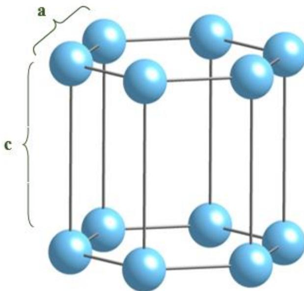
Figure 101. Bravais lattice of a hexagonal unit cell for  $\text{FeCO}_3$ ,  $\text{CaCO}_3$ , and  $\text{Fe}_x\text{Ca}_y\text{CO}_3$  ( $x+y=1$ ) [42]
