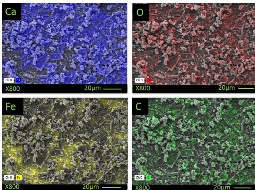
Figure 50. SEM and EDS mapping analysis of the surface layers formed during 5 days of cathodic polarization; Fe is absent in the precipitated crystalline phases ( $80^\circ\text{C}$ , bulk solution pH 5.5,  $\text{pCO}_2$  0.53 bar, 6000 ppm  $\text{Ca}^{2+}$ , 0.60 M ionic strength, and 20 rpm)
