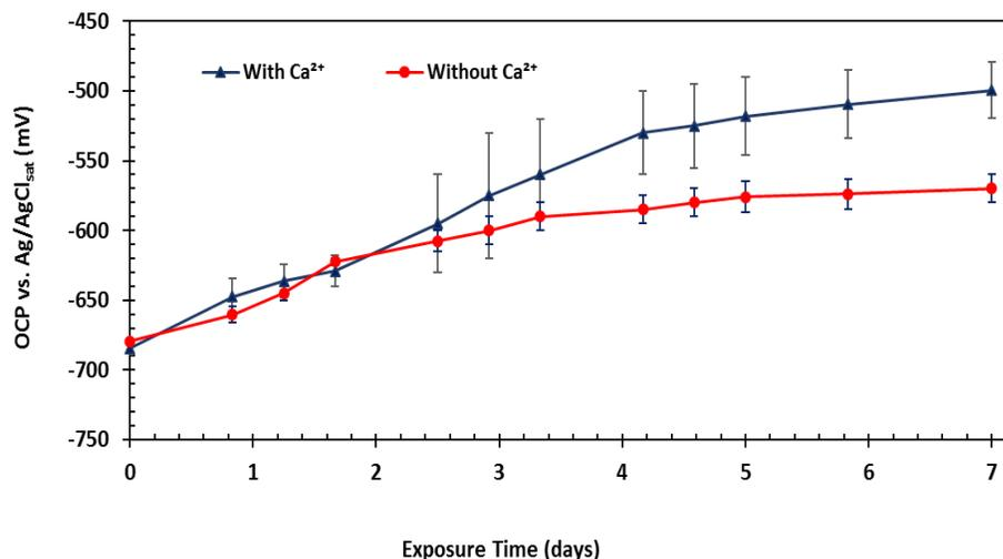
Figure 40. 5 Comparison of OCP over time for UNS G10180 exposed to solutions without and with 6000 ppm Ca<sup>2+</sup> ( $S_{CaCO_3} = 1$ ) at 80°C, pCO<sub>2</sub> 0.53 bar, bulk solution pH 5.5, 0.60 M ionic strength, and 20 rpm
