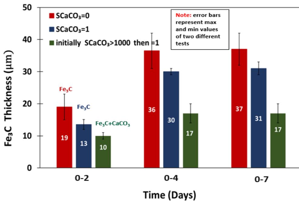
Figure 65. Fe<sub>3</sub>C growth on mild steel over time exposed to solution with different CaCO<sub>3</sub> saturation levels at 80°C, pCO<sub>2</sub> 0.53 bar, 20rpm, pH 6.2, ionic strength 0.18 M, [Ca<sup>2+</sup>] ~160 ppm
