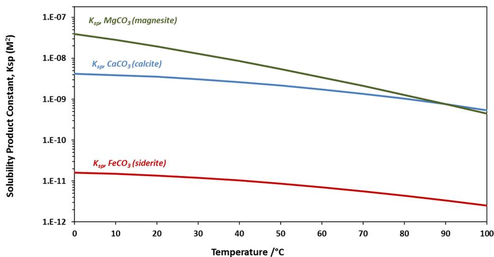
Figure 1. Solubility products of siderite, calcite, and magnesite *versus* temperature
