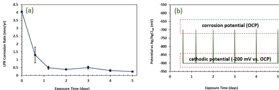
Figure 52. LPR Corrosion rate (a) and potential variations (b) over time during cathodic polarization of the specimens (80°C, bulk solution pH 5.5, pCO<sub>2</sub> 0.53 bar, 6000 ppm Ca<sup>2+</sup>, 0.60 M ionic strength, and 20 rpm)
